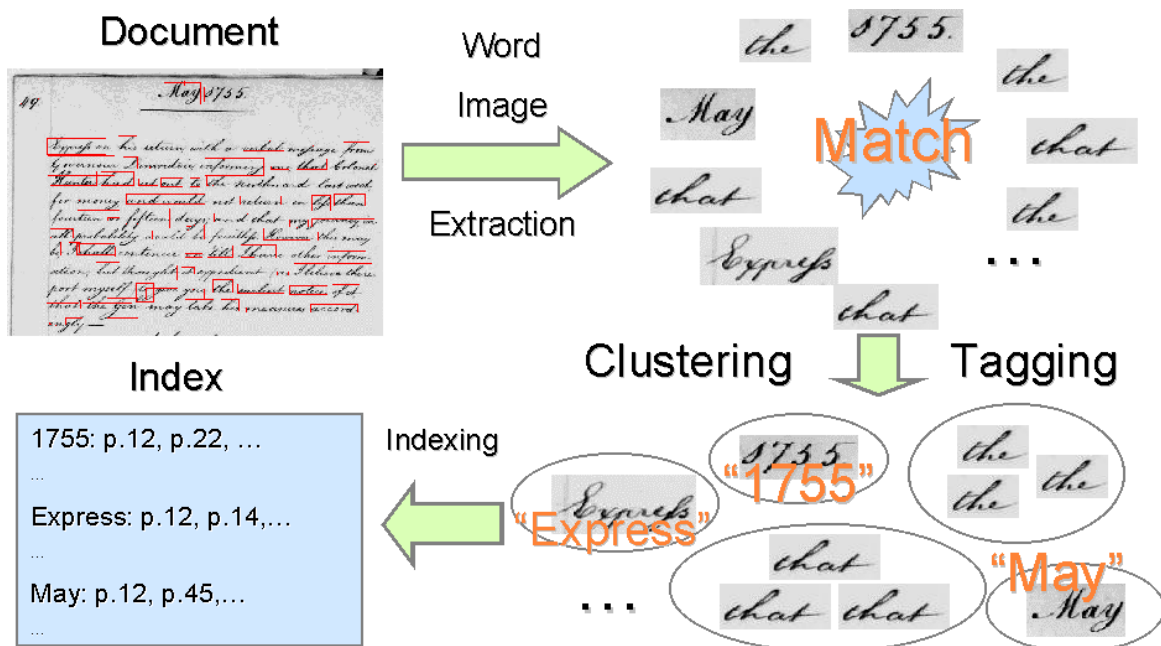
Figure 1.2: An illustration of the word spotting process. Documents are segmented and distances between word images are calculated. After clustering the word images, some clusters are manually labeled and can be used as index terms. Figure reproduced from [62].
