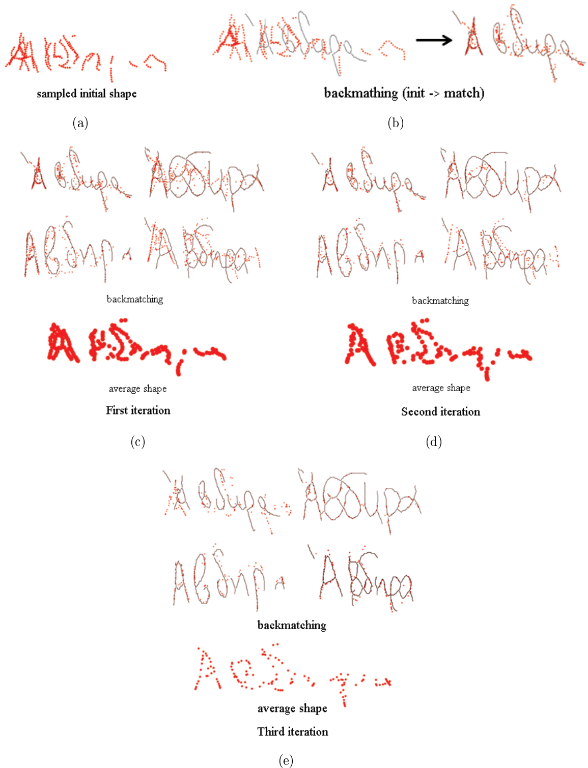
Figure 3.4: Model shape refinement. (a) Sampled points from the initial shape. (b) After initializing backmatching by aligning the model with the image bounding-box (left), the model deforms so as to match the image edgels (right). (c) The first, (d) second and (e) third iteration of shape refinement along with the corresponding average shape.
