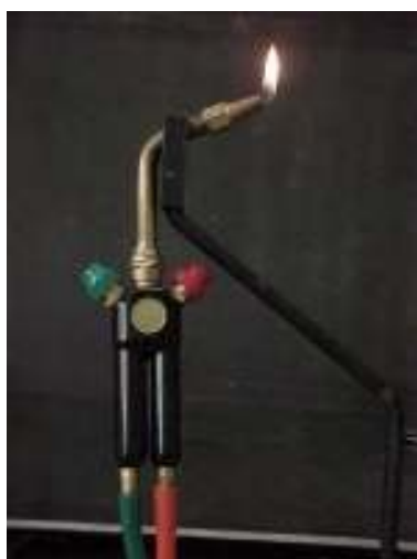
Figure 2.3: A glassblowing hand torch. The red valve adjusts gas and the green oxygen.
