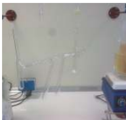
Figure 6.8: Photo of the apparatus for the purification of naphthalene, attached on the vacuum line.
