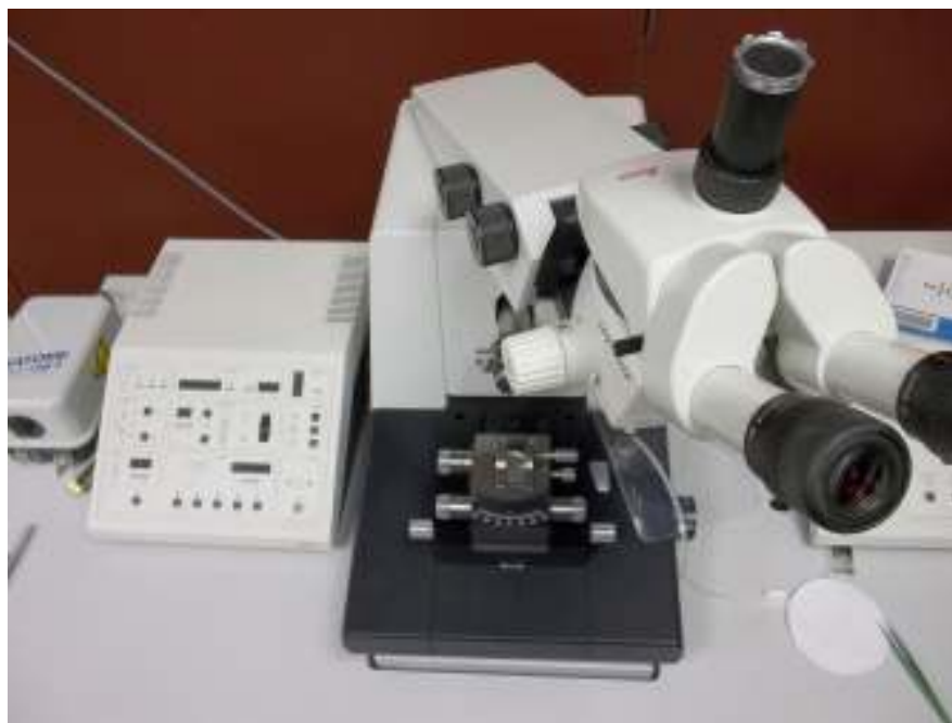
Figure 6.21: The Leica Ultracut UCT ultramicrotome used for ultra-sectioning of the samples.
