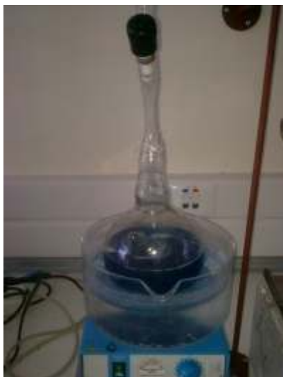
Figure 6.4: Picture of the flask with THF in Na/K alloy attached on the vacuum line.
