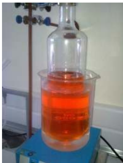
Figure 6.3: Picture of a cylinder with (polystyryl)lithium living ends in benzene attached on the vacuum line.
