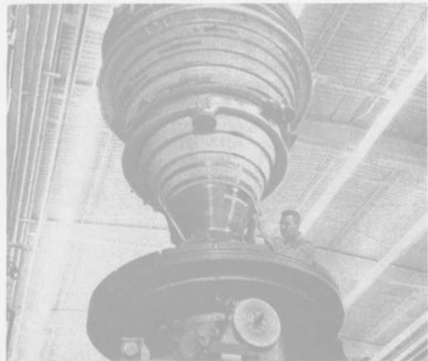
J-2 Engine. Workmen square up components of a J-2 hydrogen fuelled rocket engine at the engine thrust chamber of the Rocketdyne Plant, California, U.S.A. The J-2 is under development for the Saturn V rocket.
