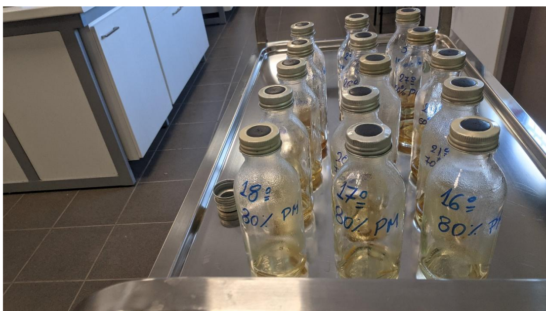
Figure 8. Glass reactors removed from the incubator after substrate pretreatment and prior to the co-digestion experiments
