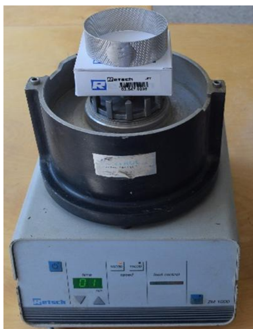
Figure 2. Laboratory mill used for milling the rice biomass with a 0.5 mm sieve
