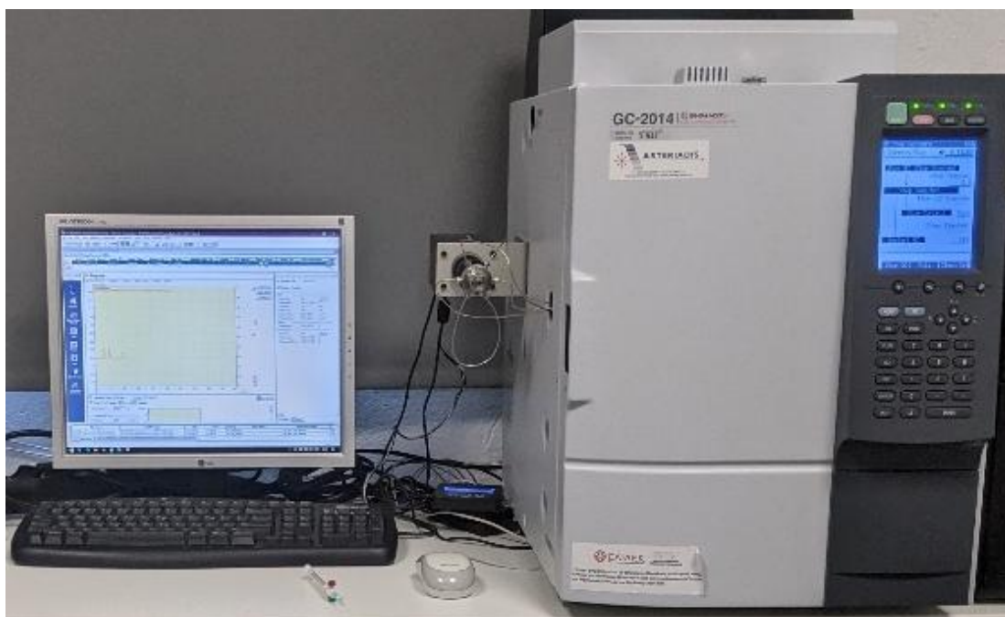
Figure 6. The Gas Chromatograph used for measuring the percentage of methane in the biogas mixture.
