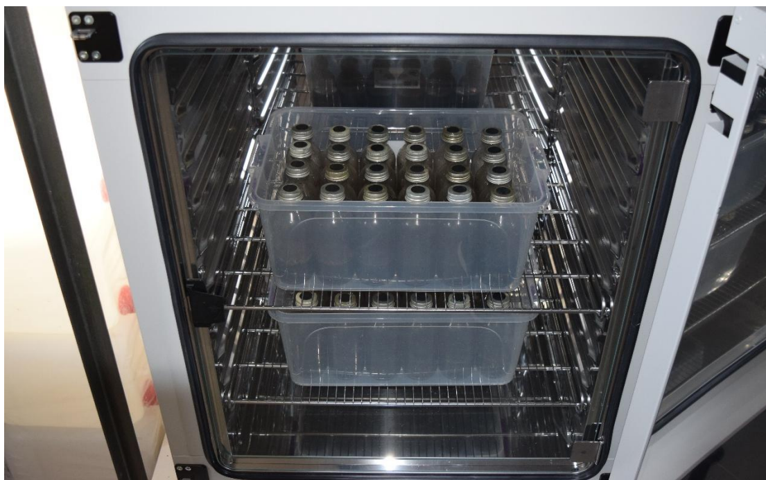
Figure 8. The glass reactors from the co-digestion experiments placed in a growth chamber (incubator) under mesophilic conditions (37 °C).
