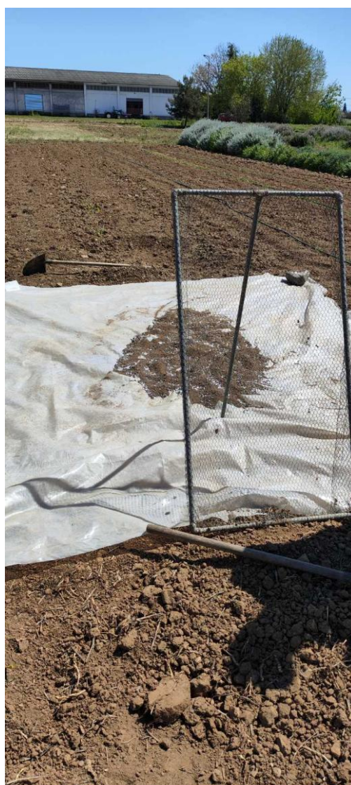
Figure 10. The methodology employed to sieve the soil with a 2 mm sieve.
