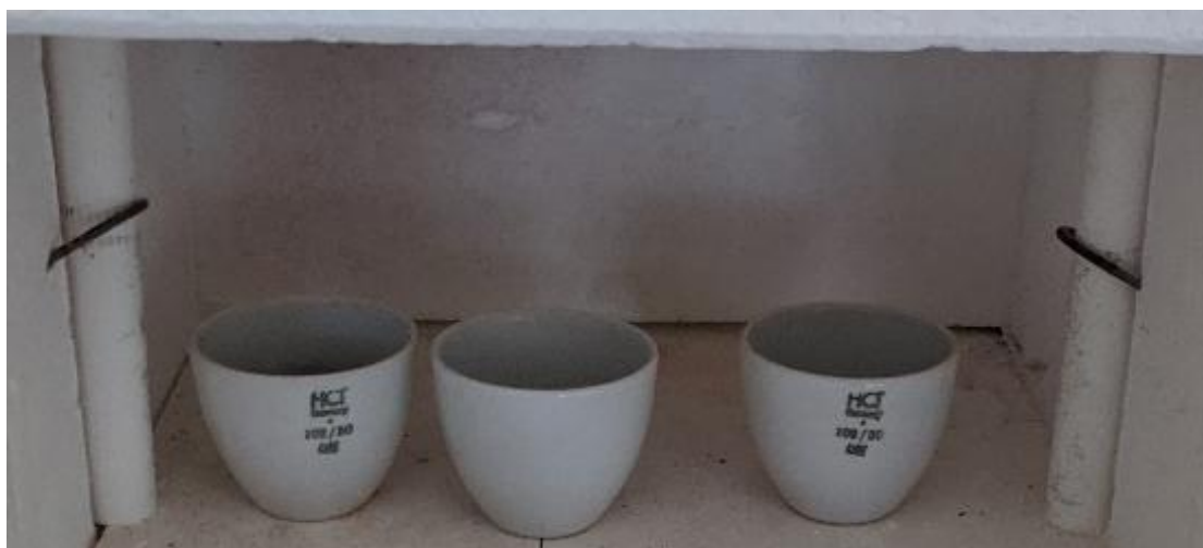
Figure 3. Crucibles placed in a muffle furnace to estimate volatile solids (VS).
