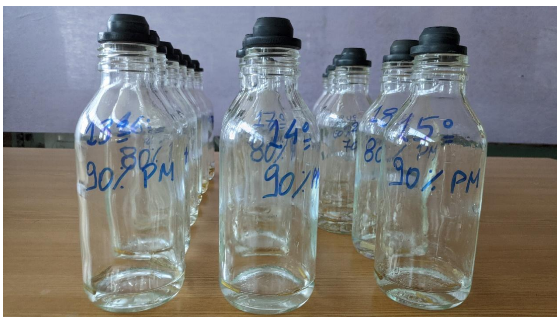
Figure 6. Glass reactors used in the co-digestion experiments
