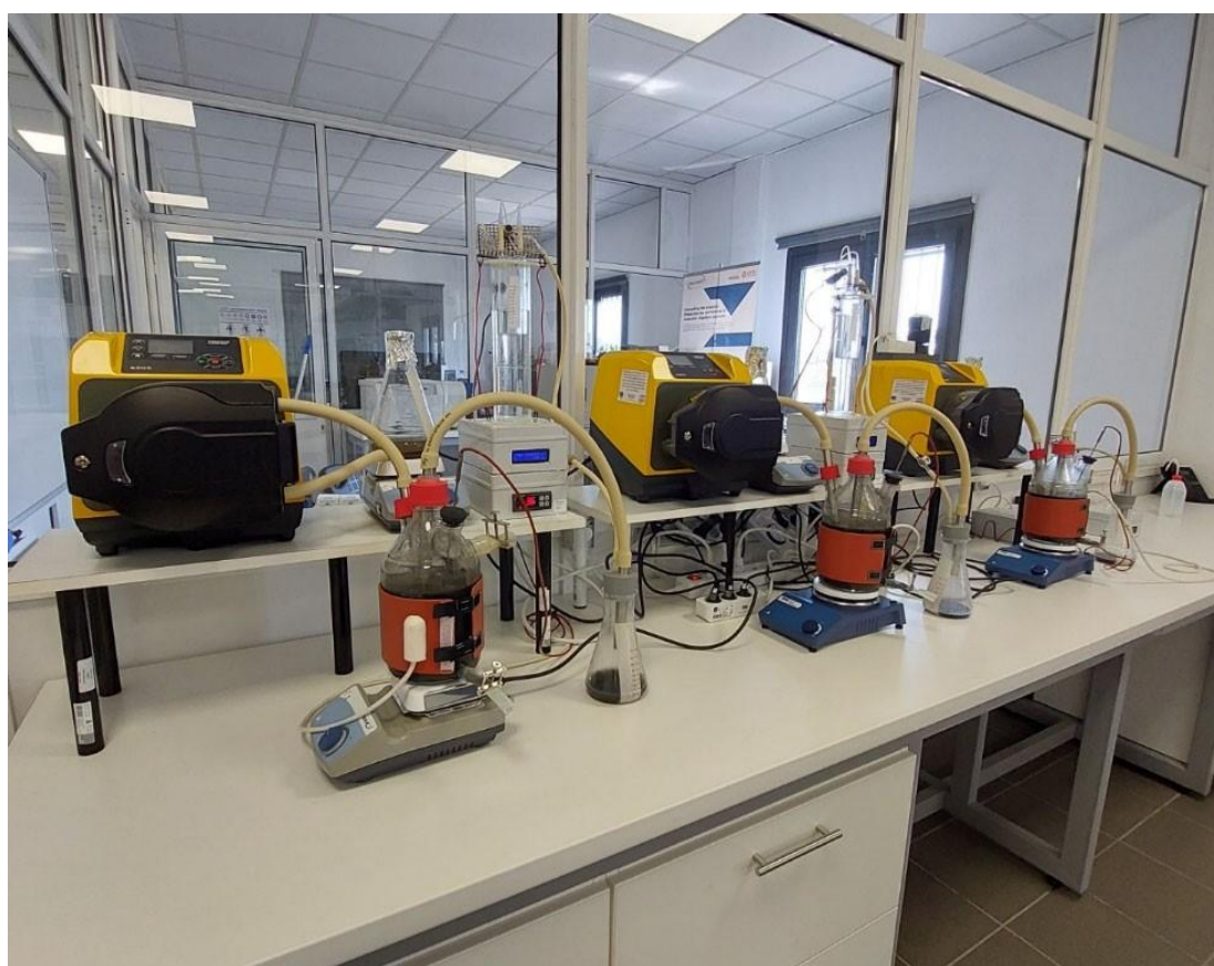
Figure 1. The three continuous stirred tank reactors (CSTR) used in the current experiment. The reactor on the left is R1, the middle one is R2, and on the right is R3.
