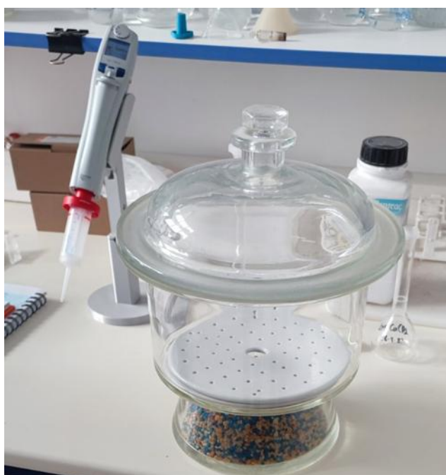
Figure 4. Portable laboratory desiccator where samples were placed after being removed from the muffle furnace.
