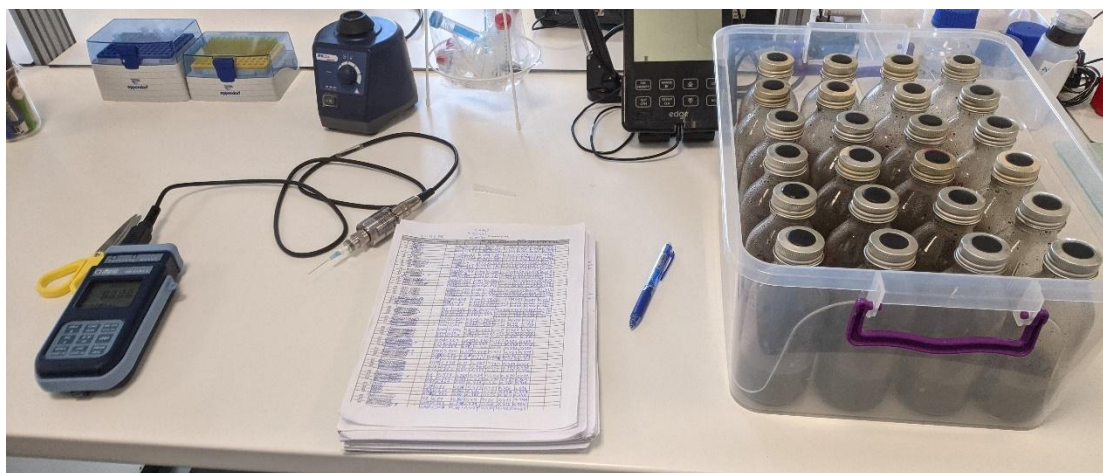
Figure 5. Glass reactors on the right and a digital manometer on the left were used to measure the pressure inside the glass reactors.
