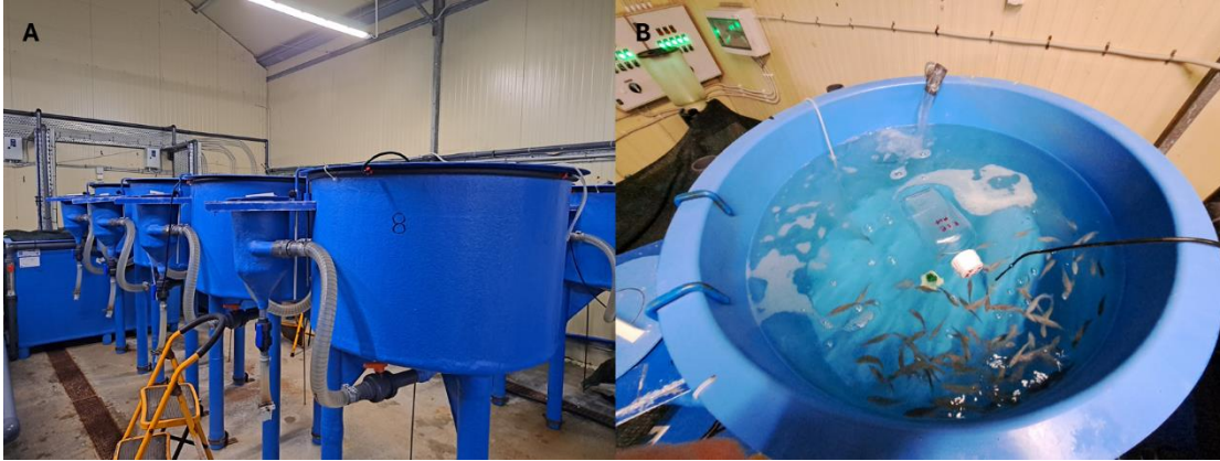
Appendix 2. Main compartments of the experimental recirculating aquaculture system operated by the Department of Ichthyology and Aquatic Environment of the University of Thessaly in Volos. A: Fish rearing tanks and biofilter. B: Fish tank with incubation bottle for the protist growth experiment.
