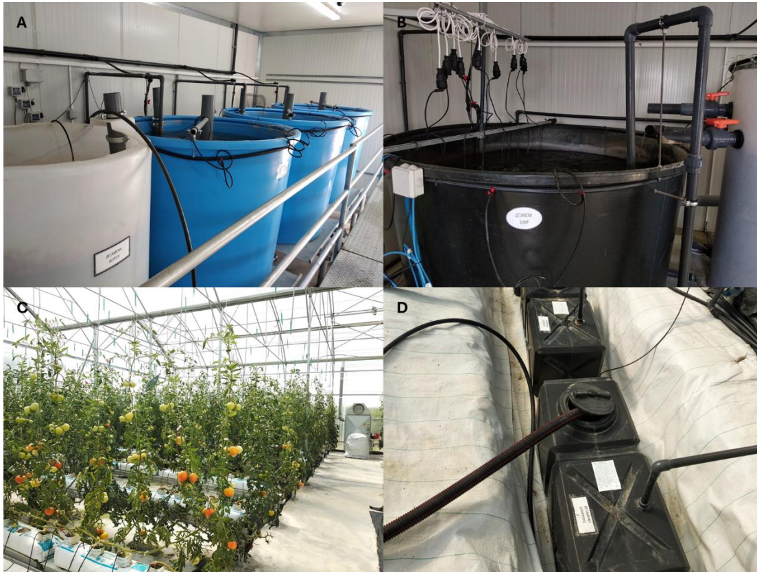
Appendix 1. Main compartments of the experimental aquaponics system operated by the School of Agricultural Sciences of the University of Thessaly in Velestino. A: Fish rearing tanks (in blue), B: sump tank, C: hydroponics compartment with tomato plants, D: drain tanks following plant fertigation.
