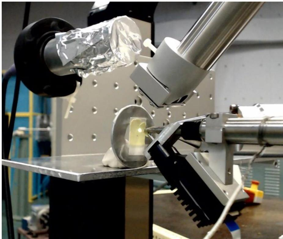
*Figure 40. Irradiation of a fluorescent ZnS sample at the intersection point of the two laser beams.*
