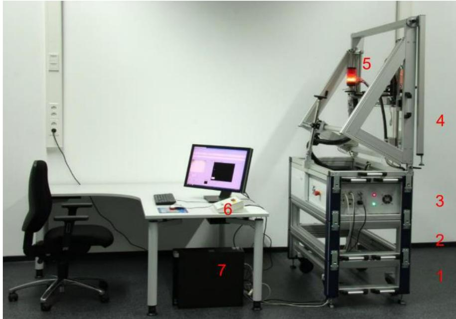
Figure 27. System components of M6 Jetstream (Bruker Nano GmbH, 2021).
