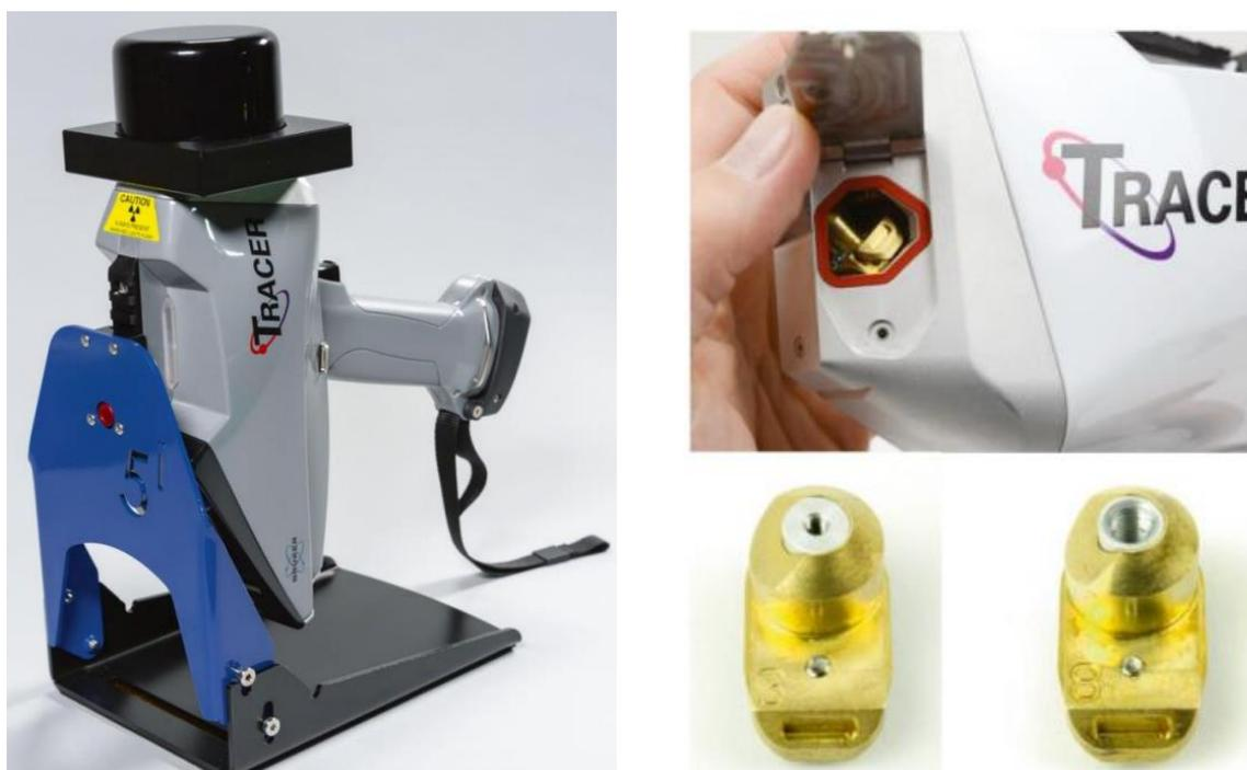
*Figure 25. Left) The HH-XRF spectrometer, Tracer 5i (Bruker) along with the benchtop stand kit and the safety cover in place. Right) The port for inserting the 3 mm and 8 mm collimators ([Bruker, 2021](#)).*
