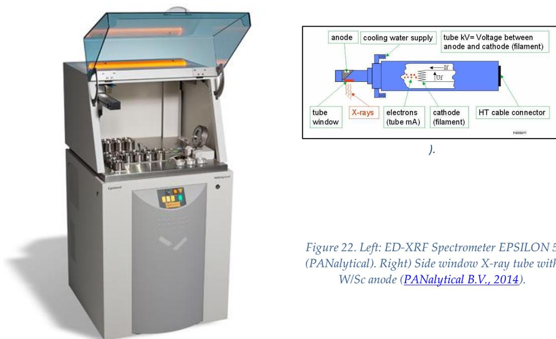
Figure 22. Left: ED-XRF Spectrometer EPSILON 5 (PANalytical). Right) Side window X-ray tube with W/Sc anode ([PANalytical B.V., 2014](#)).
