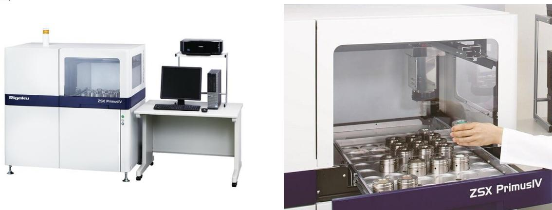
*Figure 31. Right) The ZSX Primus IV WD-XRF spectrometer. Left) Inserting samples on the WD-XRF spectrometer.*
