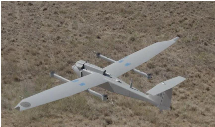
*Figure 3 AeroVironment's JUMP 20 fixed wing UAV*
