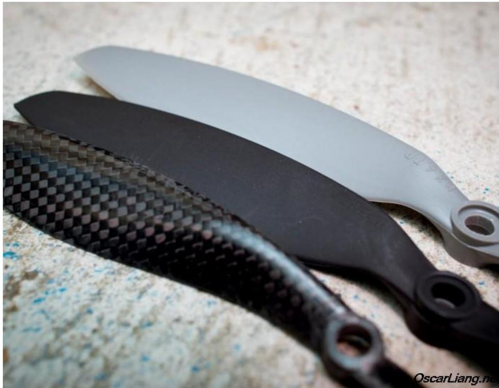
*Figure 22 Different Material Propellers*
