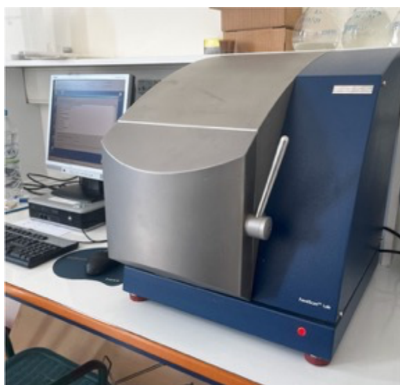
Figure 2.15. Chemical analysis of meat samples using the “FoodScan™ Lab analyzer”
