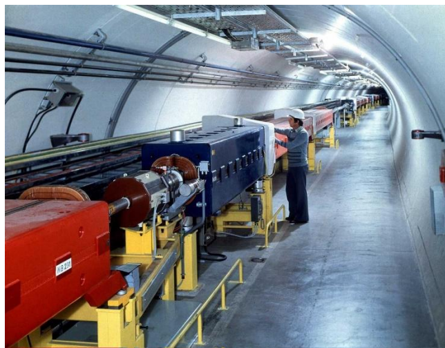
Figure 3: The Super Proton Synchrotron (SPS) facilities at CERN. The SPS, like other accelerators except the LHC, is hosted in a tunnel in the Meyrin site of the CERN facilities. In the image, there are the accelerator machine and several structures that include the beam pipe, the magnets, and the cooling system like the LHC picture above.
