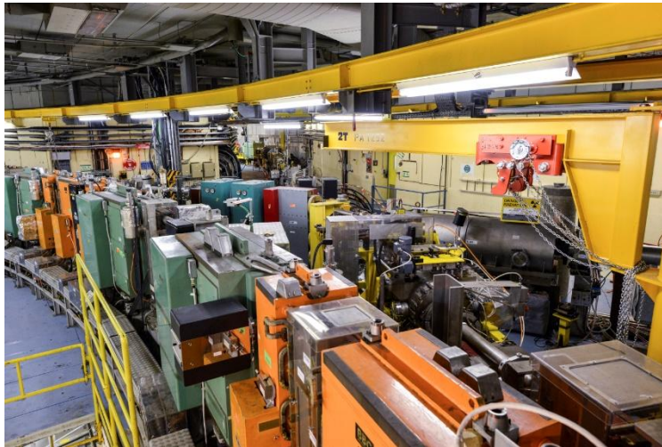
Figure 5: Picture of the Proton Synchrotron Booster (PSB) facilities at CERN. The PSB, like all other accelerators but the LHC, is hosted in a tunnel in the Meyrin site of the CERN facilities. In the image, there are the accelerator and several structures including dipole magnets (in orange), quadrupole magnets (in green), and the cooling system that all together keep the particles focused and moving on the right trajectory.
