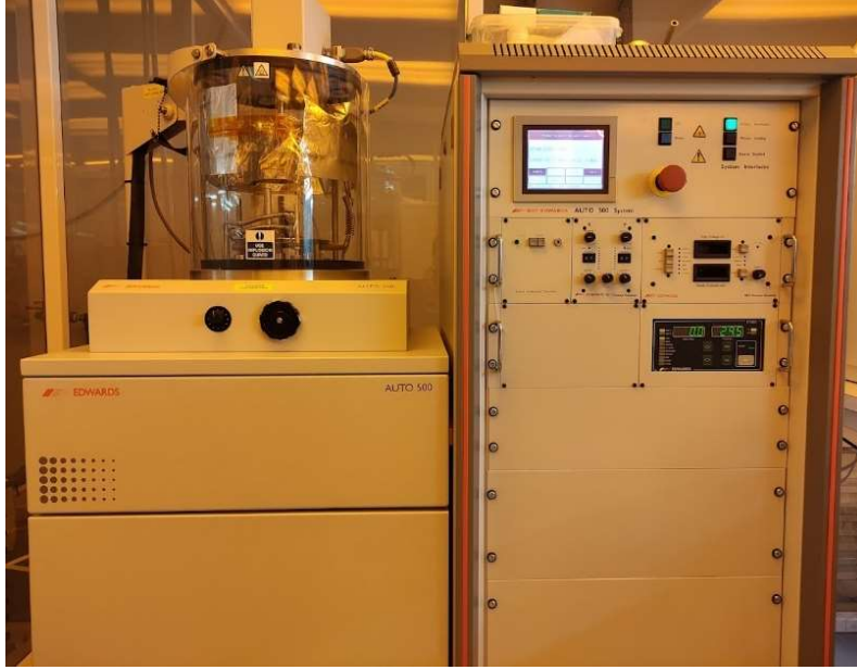
Figure 10. E-beam evaporation equipment used for fabricating contacts
