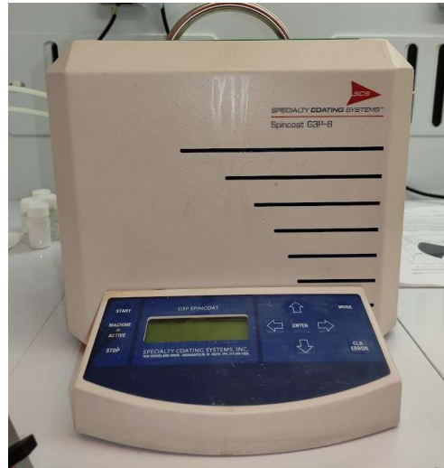
Figure 8. Spin coater used for thin film deposition
