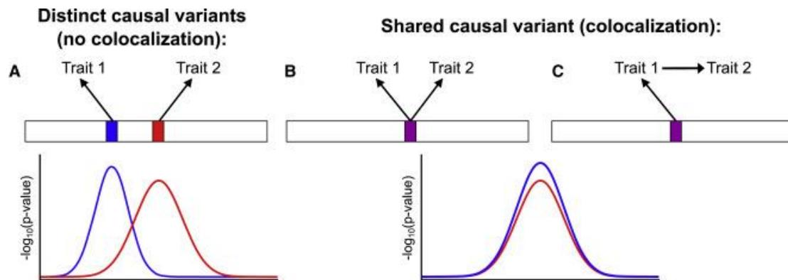
**Figure 3.2 Schematic illustration in three colocalisation scenarios**
