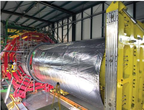
(c) The cold mass just before insertion to the cryostat barrel. In red the iron return for the solenoid and for an intersection of yoke in the CMS barrel region. [10].
