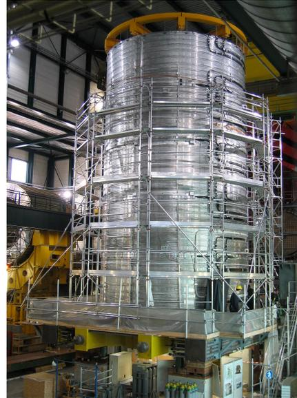
(b) The cold mass in its entirety with thermal shields [2].
