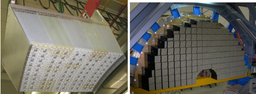
(a) Barrel 500-module mounted with all crystals.
