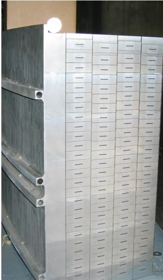
(a) The cold mass four-layer  $NbTi$  coil-winding [10].
