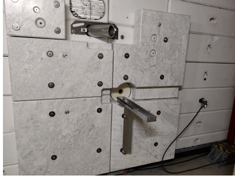
Figure 17: An overview of a-NEAR. The outermost layer of the target bunker shielding, a 200mm thick layer of marble and the Aluminium supporting rail can be seen.
