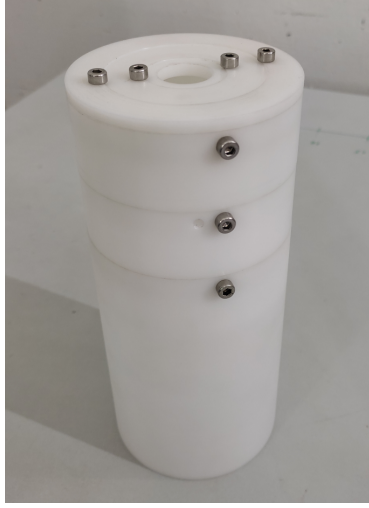
(a) Spacers to achieve different sample-to-detector distances
