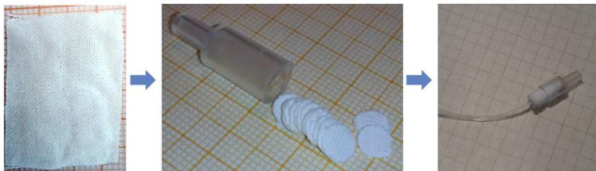
Figure 1.9.1.5 Configuration of on-line flow injection fabric disk sorptive extraction (FI-FDSE) with permission of Elsevier[450].
