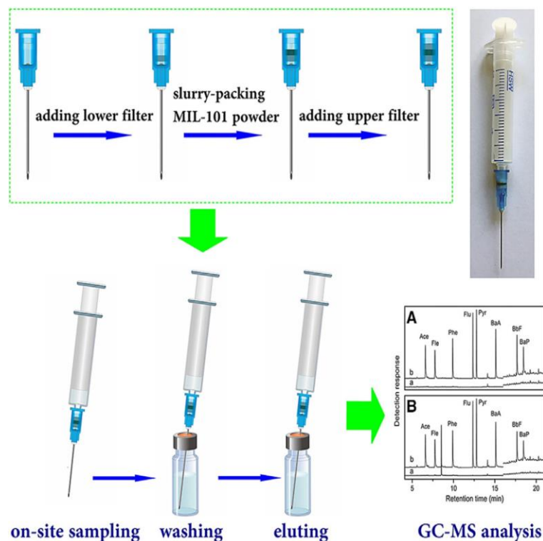
Figure 1.7.5.1 Diagram outlining the preparation process for the MIL-101-based in-syringe solid-phase extraction (SPE) device and its practical use in on-site sampling[195].
