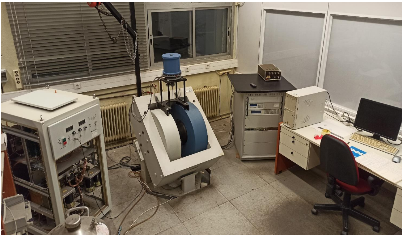
Figure 2.13 Conventional Vibrating Sample Magnetometer setup, Lake Shore Cryotronics model 7300.
