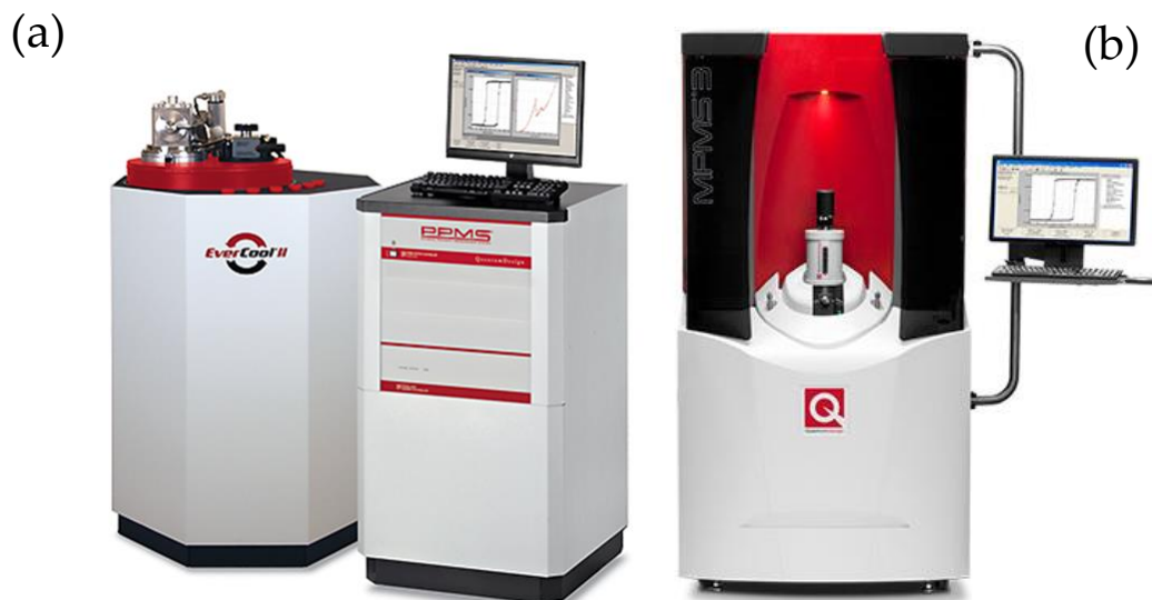
Figure 2.14 Physical Property Measuring System equipped with an EverCool II dewar option (a) and Magnetic Property Measurement System devices (b) (Quantum Design).
