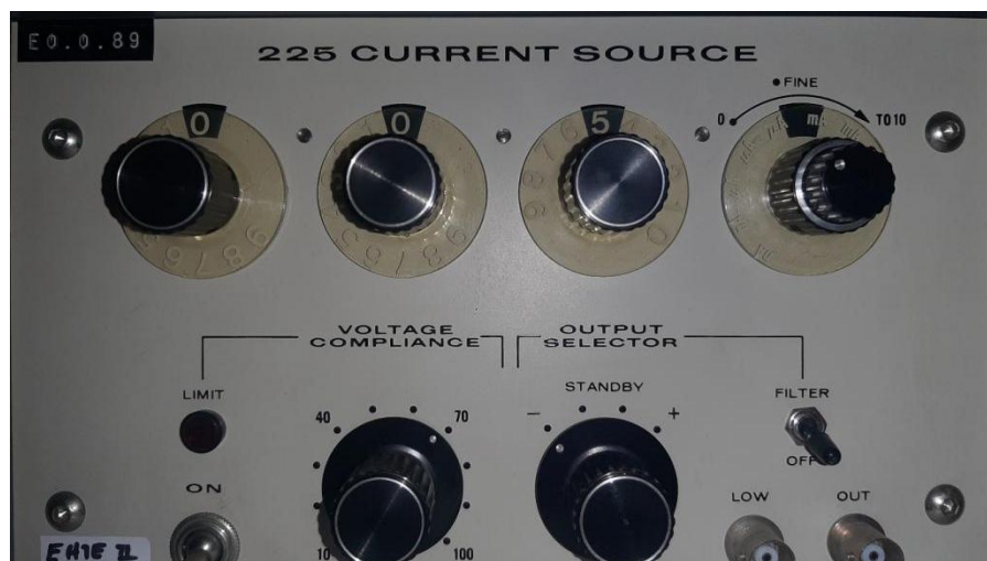
Image X: KEITHLEY 225 Current Source.
