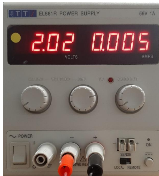
Image IX: TTi EL561R Power Supply.
