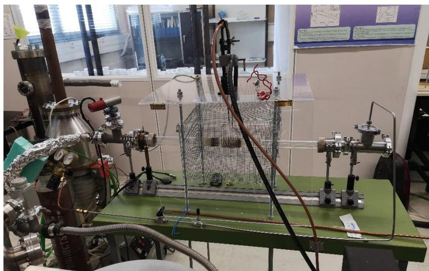
Figure 40: Oxygen plasma setup of post-growth thin film treatment.
