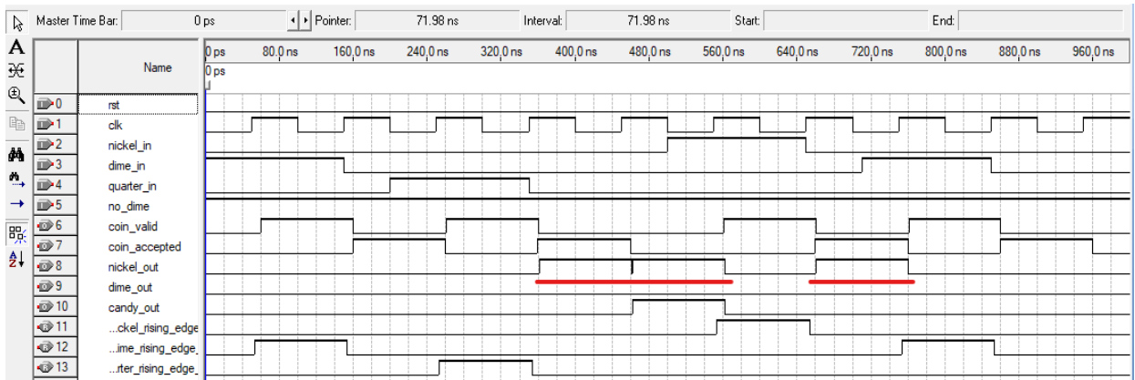
Εικόνα 39 Simulation when quick coin insertion is made and no dime is enabled.vwf
