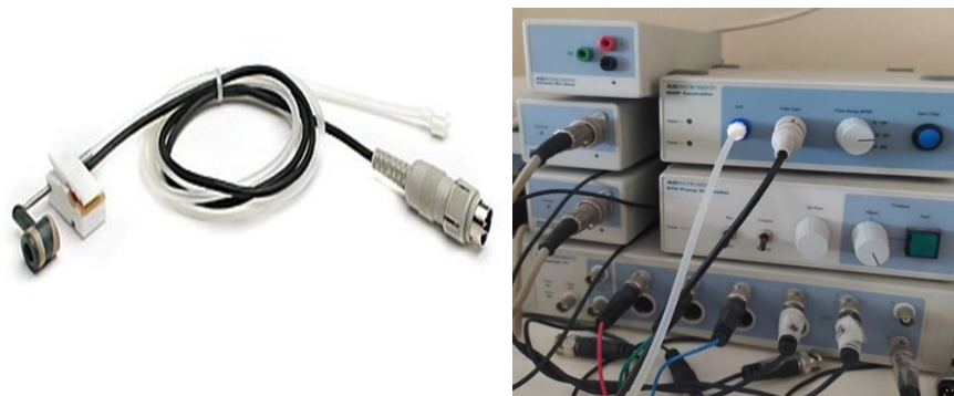
Figure 16: (Left) Tail cuff, (Right) Non-invasive Blood Pressure System for mouse or rat (NIBP System, ADInstruments Inc.)
