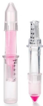
Εικ. 36: Φίλτρα Amicon Ultra-2 Centrifugal Filter Devices (for volumes up to 2 mL)
