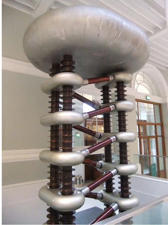
Figure 1.1: The Cockcroft-Walton accelerator terminal in the Grand Gallery at the National Museum of Scotland. Taken from [1].
