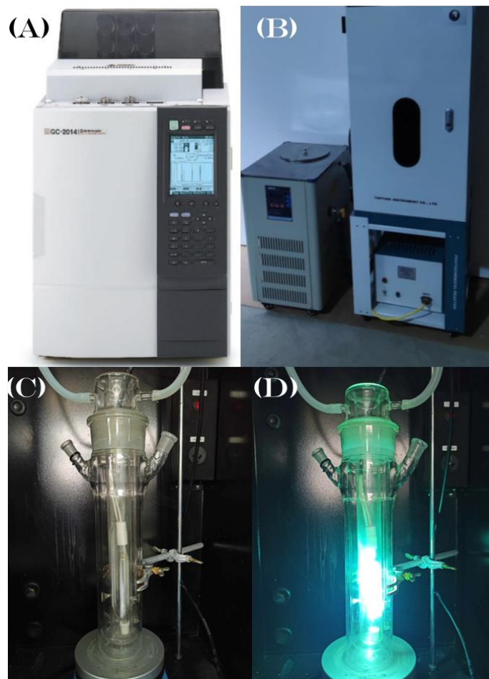
Figure 3-6: (A) The Gas chromatography system of the experiments, a TCD- Shimadzu GC-2014, with a Carboxen 1000 column. (B) The Chiller T-300W and TOPT-II photo reactor container. (C) The double-walled photoreactor. (D) The same Reactor under the illumination of the 300W Mercury Lamp.
