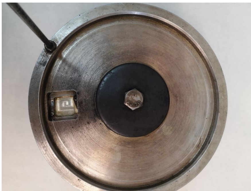
Figure 2.9 Watercooled holder of FSP-FILM Set-Up with 10 spots available.
