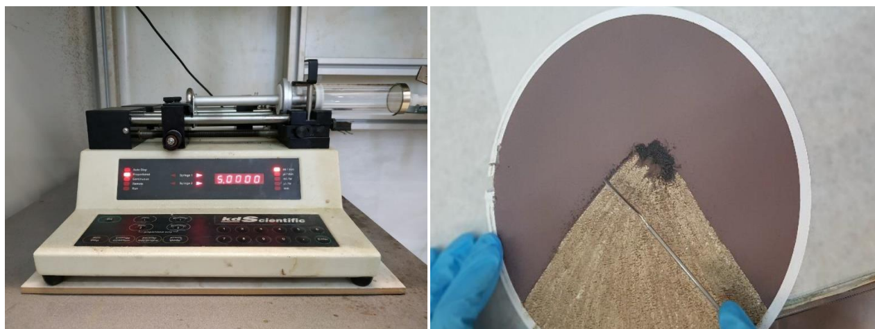
Figure 2.6 On the left the FSP atomizer, on the right the glass fiber filter in collection process.
