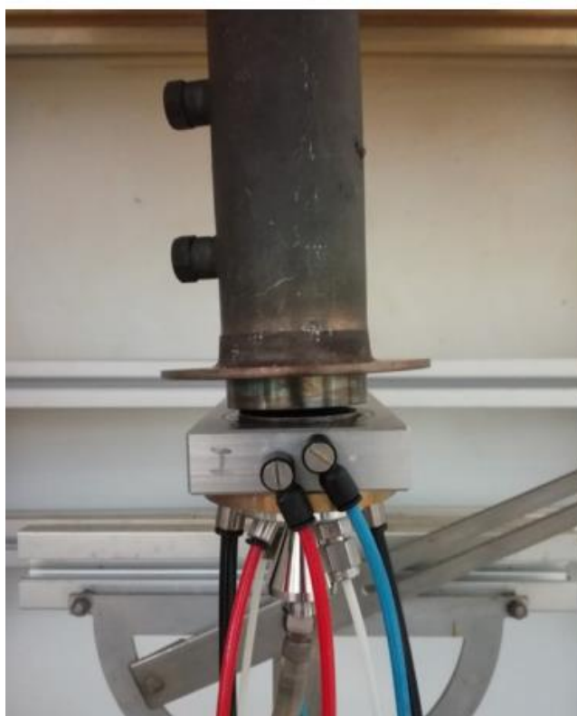
Figure 2.9: Photograph of the metallic tube at 1 cm above the FSP-nozzle in order to increase the High-Temperature Residence Time.
