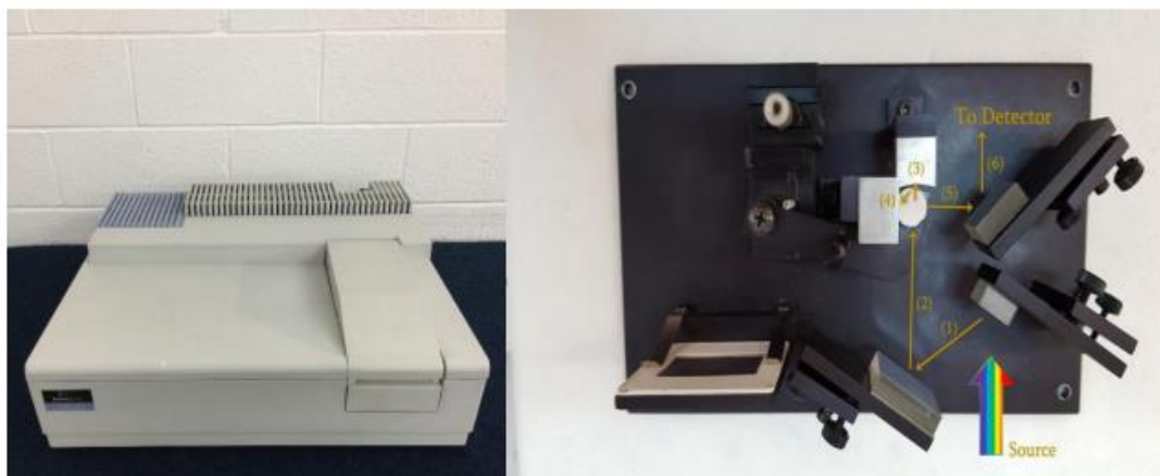
Figure 2.21: Photograph of the Perkin Elmer Lambda 35 spectrophotometer (left). The optical beam path inside the apparatus (right).
