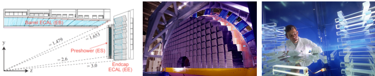
Figure 3.8: Geometric view of one quarter of the ECAL [20], crystals of half the Endcap of ECAL (center) [23] and lead tungsten crystals (right) [24].
