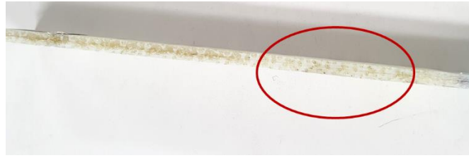
Figure 111. Composite specimen after the healing process with squeezed BMI film at its edges.
