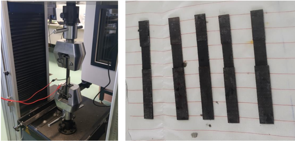
Figure 69. Mechanical testing process of lap strap specimens with online impedance measurements (left) and lap strap specimens (right).
