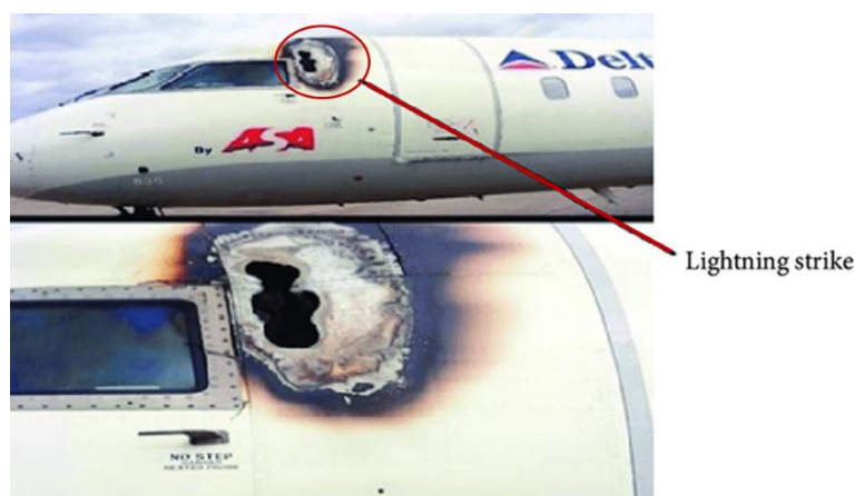
Figure 5. Damage occurred from a lightning strike at aircraft.
