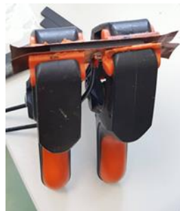
Figure 9. Experimental configuration of IS measurements of SENB specimens.
