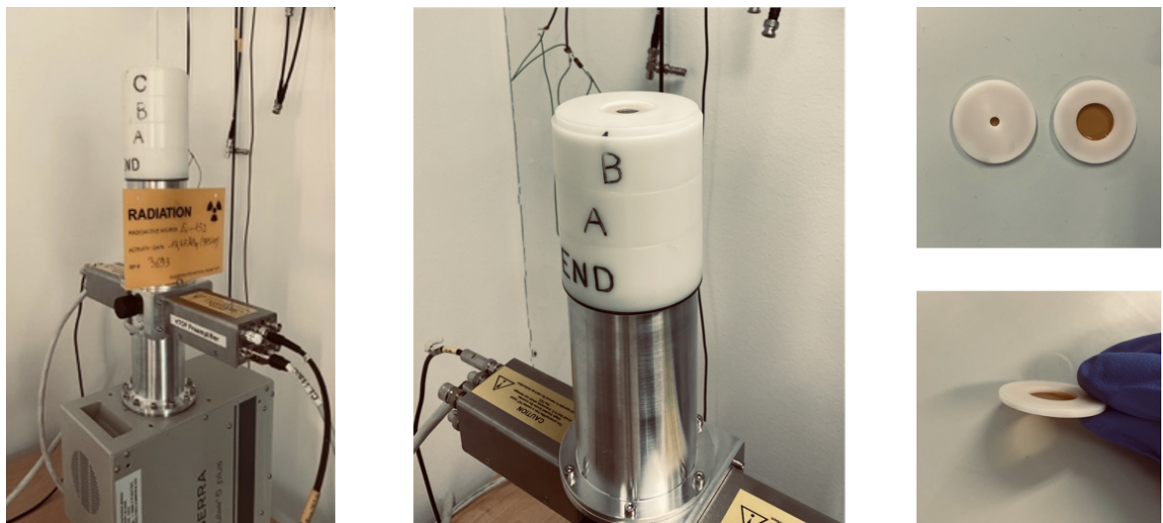
FIGURE 2.7. The HPGe detector at n_TOF/CERN along with polyethylene spacers and rings.
