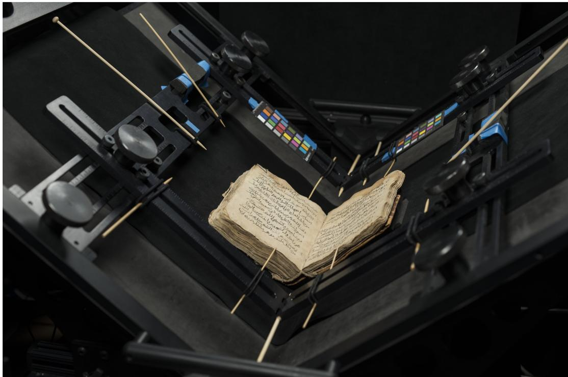
*Note.* Glass platen that flattens pages of manuscript is removed and replaced by EMEL manufactured aluminum frame
