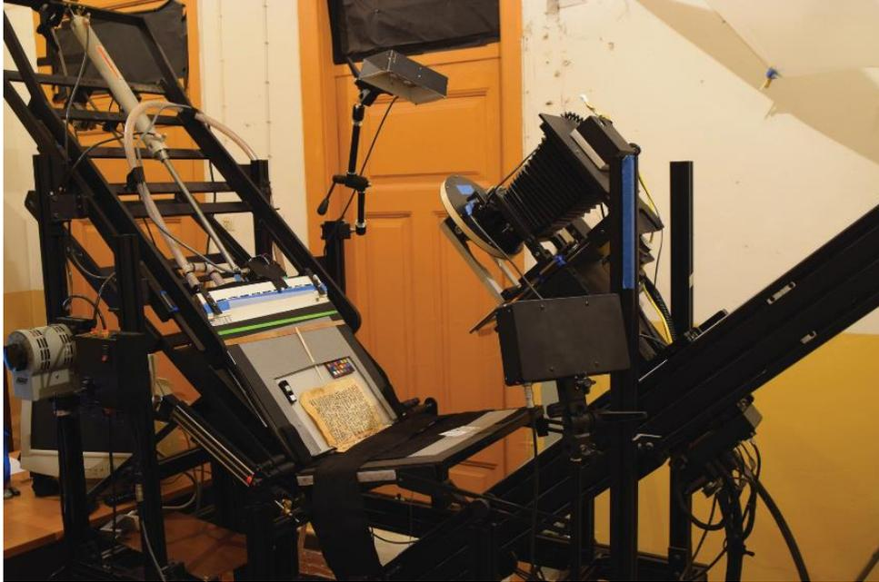
*Note.* Camera, lens and filter wheel on right side, manuscript and calibration targets on left side of photograph
