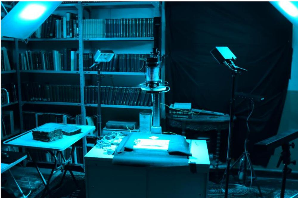
Note. Camera, lens, filter wheel in the center, manuscript rests flat below camera, lights on the right and left illuminating with cyan light the object
