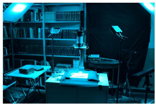
Spectral imaging system on copystand setup
