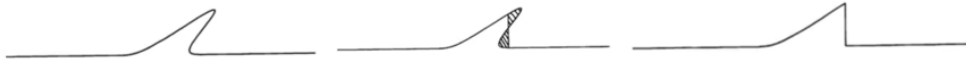
Figure 4.3: [A] Application of the equal-area principle. The shock curve is positioned in a way that A1=A2 . [B] The stages of shock formation through the equal-area approach.
