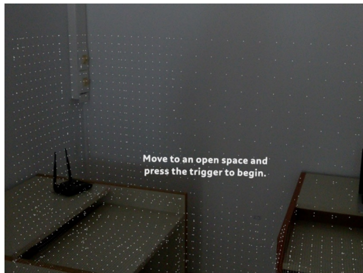
Figure 40. The AR device displaying spots in the physical environment to recognize the space. The participant should look at different directions and move in order the space to be recognized
