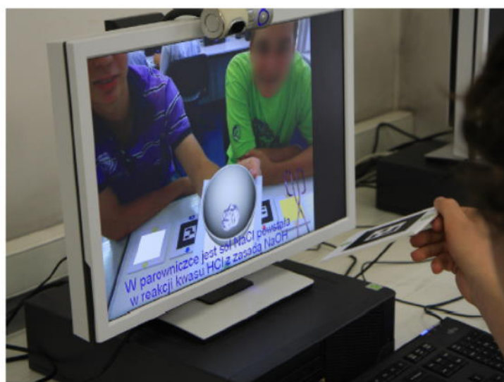
Figure 3. AR installation – a desktop PC with a monitor, a webcam, a set of physical markers
