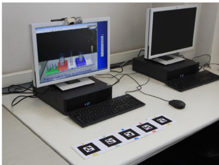
Figure 3. AR installation – a desktop PC with a monitor, a webcam, a set of physical markers
