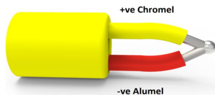
Figure 57: A schematic of a type-K thermocouple as the one we constructed for that EPR set-up.
