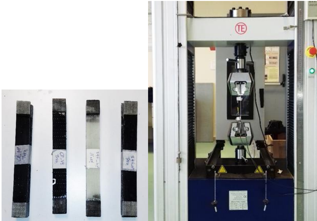
Figure 2-15 GFRP tensile specimens with neat and ternary modified epoxy matrix (left) and the tensile testing machine (right).
