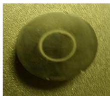
Figure 2-4 Sliding wear rate specimen shape and dimensions (left) and the CSM ball-on-disk tribometer apparatus (right).
