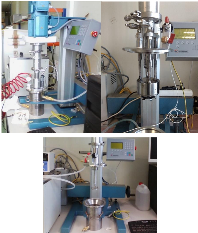
Figure 2-1 Dissolver Dispermat mixer (top left), the bead mill module (top right) and the impeller disk module (bottom).
