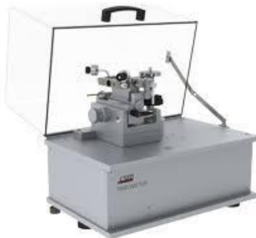
Figure 2-4 Sliding wear rate specimen shape and dimensions (left) and the CSM ball-on-disk tribometer apparatus (right).
