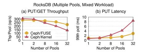
Figure 3.5: Limited multitenant isolation. This figure depicts the limited I/O isolation shown by the decreasing throughput and increasing tail latency per pool of RocksDB over the Ceph storage.
