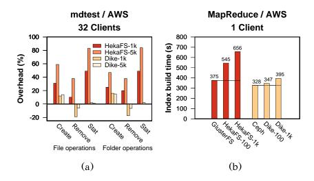
Figure 11.7: **Comparison of multitenancy overheads in AWS.** This figure summarizes the comparison of relative overheads by Dike over Ceph and HekaFS over GlusterFS in the filesystem throughput of (a) mdtest with up to 5,000 tenants and (b) MapReduce with up to 1,000 tenants.
