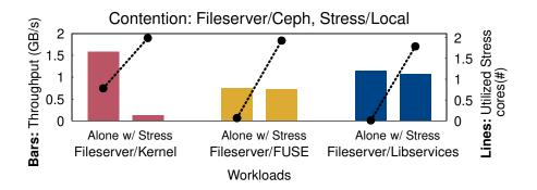
Figure 4.3: **Sensitivity to neighbor noise**. The performance of the kernel Ceph client is sensitive to contention with the Stress noisy neighbor.
