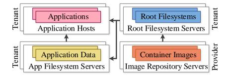
Figure 3.2: The container storage systems. The tenant applications run in containers that depend on two storage systems: (a) The Root Storage System for access to the root filesystem tree, and (b) the Application Storage System for access to the application data. The Image Repository is a third storage system that is used by the Root Storage System for access to the container images.
