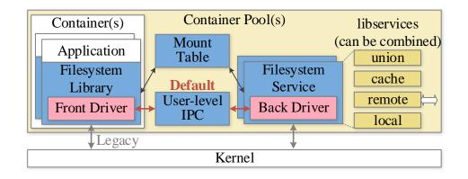
Figure 5.1: **The Polytropon toolkit.** In a container pool of Polytropon, the filesystem library communicates with the filesystem services through the mount table and the user-level IPC (default) or the kernel (legacy).
