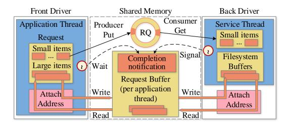
Figure 5.4: **The Polytropon IPC.** In the Polytropon IPC, the front driver transfers to the back driver small items over a request queue (RQ) and large items over a request buffer (per application thread).
