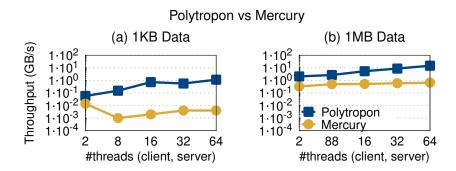
Figure 5.7: **Polytropon vs Mercury**. This figure compares the performance of the Polytropon IPC with Mercury RPC framework. On a machine with 2, 8,16, 32 or 64 enabled cores, we set both the client and server threads equal to the number of cores.
