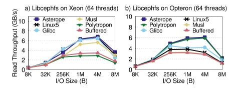
Figure 9.2: **Read I/O performance of libcephfs**. This figure depicts the read I/O performance of libcephfs over Ceph. The libcephfs that uses the memcpy routine returned by the Asterope algorithm tracks or improves the performance of the fastest memcpy routine on both systems.
