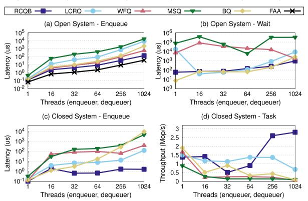
Open & Closed systems on AMD Opteron with separate threads for enqueue & dequeue
