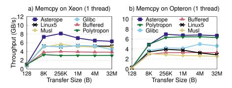
Figure 9.1: **Standalone copy throughput**. This figure depicts the copy throughput across 6 memcpy routines and 2 cpus. Asterope achieves the best possible performance on both systems.
