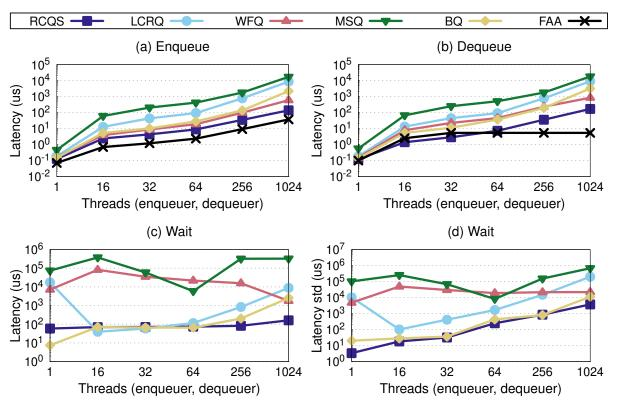
Open system on AMD Opteron with separate threads for enqueue & dequeue
