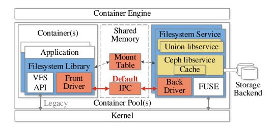
Figure 6.1: Architecture of the Danaus user-level client. The color shades illustrate the new components of Danaus and the white background the components of existing systems.
