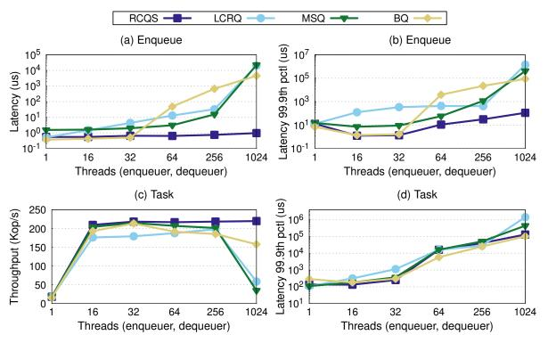
Closed system with separate threads for enqueue & dequeue (random number of nops as service)
