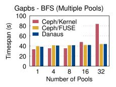
Figure 6.5: **Gapbs BFS workload**. Timespan to start and run containers with the Gapbs workload.
