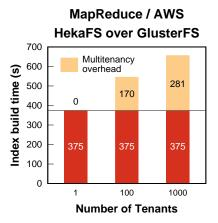
Figure 10.2: **Identity mapping overhead.** This figure shows the overhead of identity mapping added by HekaFS over GlusterFS for multitenancy support. For 1 tenant we use vanilla GlusterFS.
