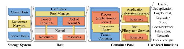
Figure 4.1: **Per-tenant storage provisioning.** The container pool of a tenant uses dedicated filesystem services built from user-level libservices. The figure depicts that the same design pattern can be used both at the client hosts that accommodate the application containers of a tenant and at the server hosts that accommodate the service containers of a tenant-provisioned distributed storage system.
