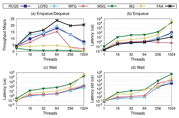
Open system with pairs of enqueue & dequeue operations per thread
