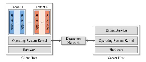
Figure 3.3: **The legacy cloud stack.** In existing systems, the containers of different tenants typically run on the shared operating system of the client machine and access shared remote services over the datacenter network.
