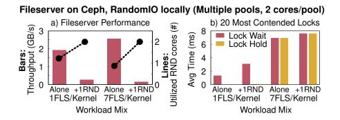
Figure 3.4: **Shared kernel contention**. This figure depicts the dramatic drop of the Fileserver throughput due to the core (a) and lock (b) contention inside the shared host kernel.
