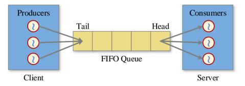
Figure 7.1: **Producer-Consumer communication.** A number of producer threads of a client process place requests on the tail of a FIFO queue. Each consumer thread of a server process extracts a request from the head of the queue and serves it.
