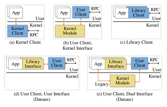
Figure 5.2: Filesystem types. Three existing types of filesystems (a-c) and two that we introduce with Polytropon (d-e).
