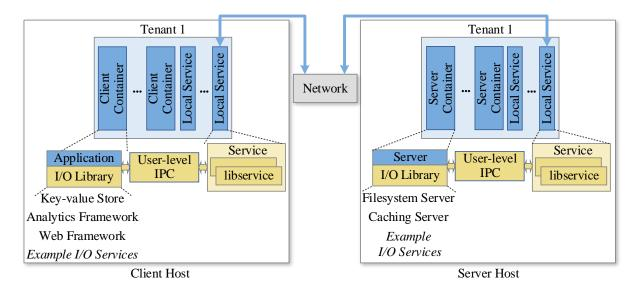
Figure 3.7: **Tenant storage provisioning.** At both the client and server side over the datacenter network, a tenant runs its own containers, interprocess communication, and local services at user level.
