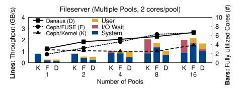
Figure 6.11: **Random I/O scaleout.** Performance and core utilization of the Filebench Fileserver at multiple pools.
