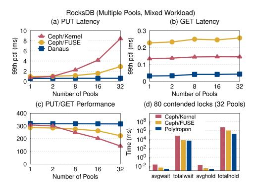
Figure 6.3: **RocksDB in scaleout setting.** The RocksDB storage engine running over three alternative Ceph clients. We measure the 99%ile of put (a) and get (b) latency, the average put/get throughput per pool (c), and the average/total lock wait/hold time (d).
