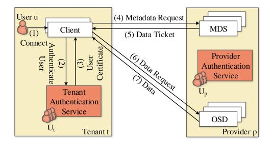
Figure 11.3: **Steps for file access in Dike.** Steps for file access in Dike. Over lines in the parentheses we enumerate the steps of file access by a user in the Dike multitenant access-control system. Important steps required for the attestation and authentication of the system nodes are omitted for readability. The new entities of Dike are denoted with dark background.
