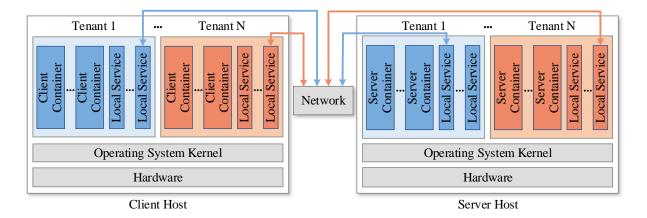
Figure 3.6: **Per tenant user-level filesystems.** In our solution, for performance and security isolation each tenant uses its own containers and local user-level services at both the client and server side inside the datacenter.
