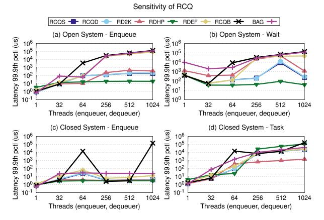
Figure 8.7: Sensitivity analysis of RCQ variants in open and closed system. Enqueue and wait or task latency 99.9%ile for open and closed system (NULL service) with 1-1024 threads (#engrs=#degrs).
