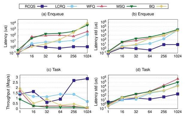
Closed system on AMD Opteron with separate threads for enqueue & dequeue
