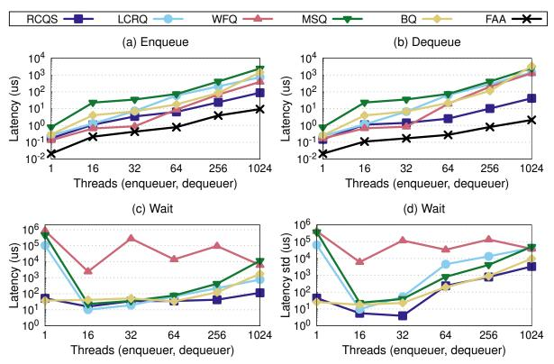
Open system with separate threads for enqueue & dequeue
