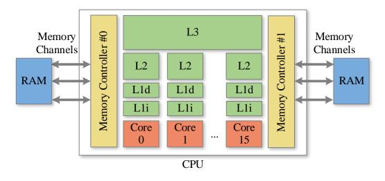
Figure 7.2: **The memory subsystem**. A memory controller is typically integrated on the CPU and communicates with the RAM modules through multiple memory channels. To access data fast, the CPU maintains a cache hierarchy that contains least-recently-used data.
