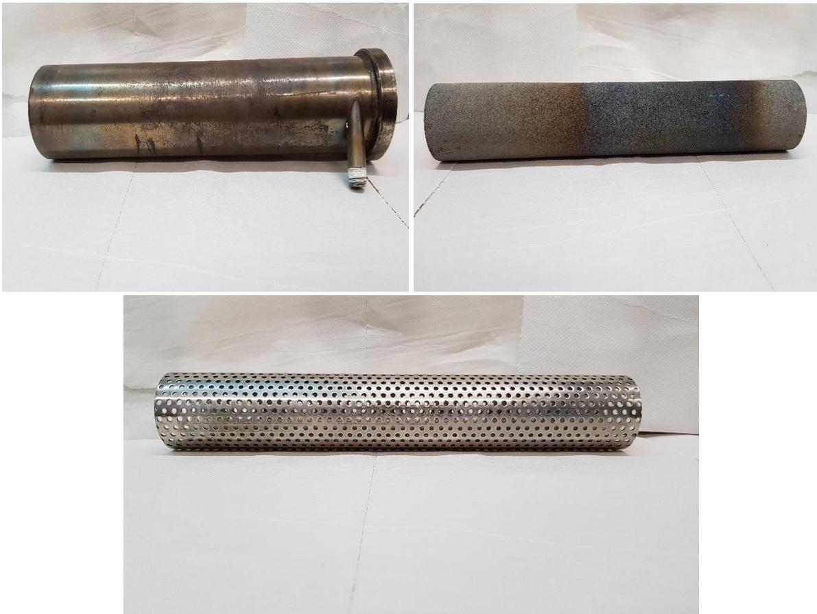
**Figure 2.39.** (Top Left): Metal sinter tube for the anoxic FSP configuration. (Top Right): Porous inner tube. (Bottom): Perforated inner tube.
