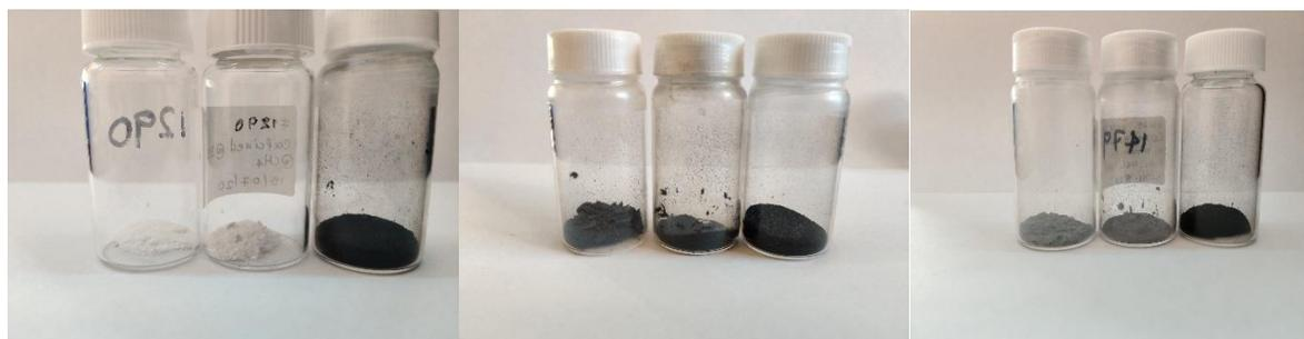
**Figure 3.2.** Left: From left to right material 1290 and upon calcination at 350°C and 800°C under CH<sub>4</sub> atmosphere, respectively. Middle: From left to right material 1323 and upon calcination at 350°C and 800°C under CH<sub>4</sub> atmosphere, respectively. Right: From left to right material 1479 and upon calcination at 350°C and 800°C under CH<sub>4</sub> atmosphere, respectively.
