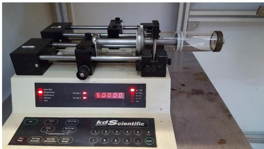
Figure 2.37. Atomization device. The precursor is converted into micron-sized droplets and sprayed with the aid of a syringe pump.
