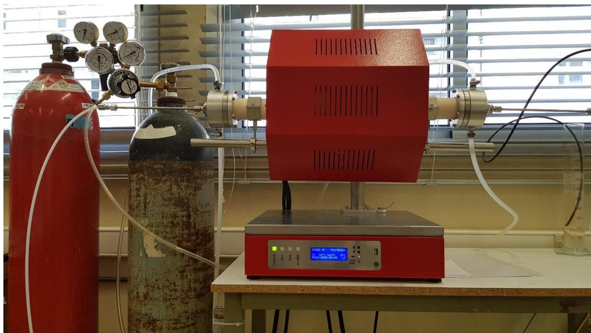
**Figure 2.22.** Thermansys 30802 tubular furnace used for calcination of samples.
