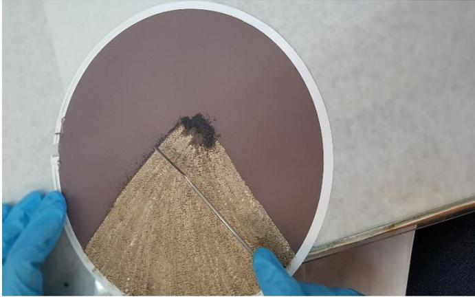
**Figure 2.38.** Particle collection. Nanopowders are collected in a glass fiber filter.
