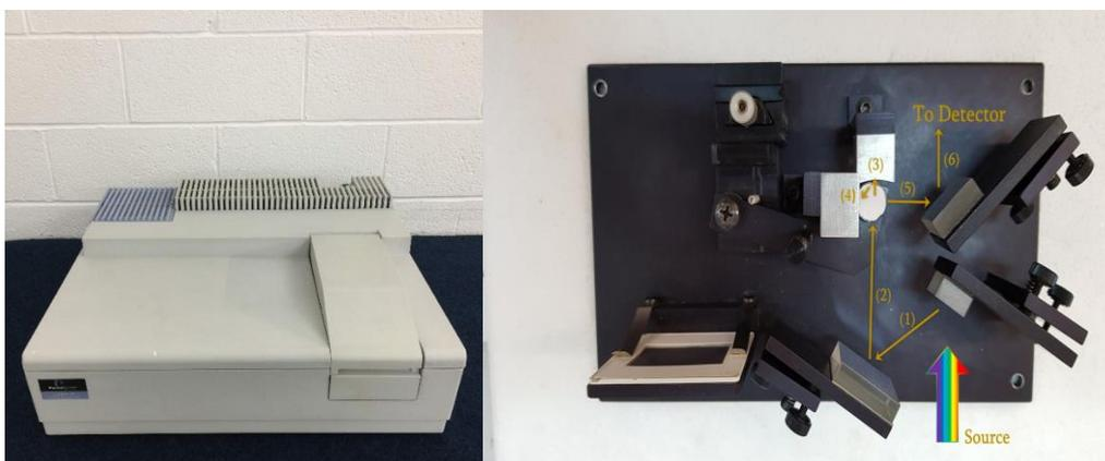
**Figure 2.14.** (Left): Perkin Elmer Lambda 35 spectrophotometer. (Right): Beam path inside the DRS.
