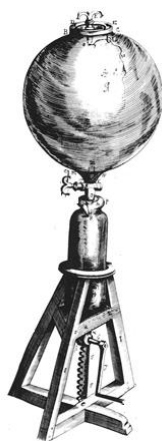
Figure 8.7: Boyle' first air-pump, with the glass receiver attached on a wooden stand
