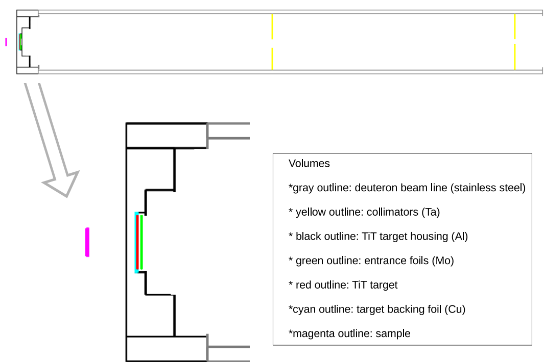
Figure 3.12: The GEANT4 visualization of the deuteron beam line and the TiT target in the accelerator facility at “Demokritos”, using the DAWN visualization driver.
