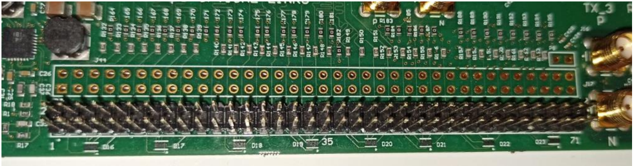
Figure 91. The pin-header connectors on the board. Only the single-ended connector is populated here. Note the series resistors above the pin header connectors and the ESD protection diodes below the connectors.
