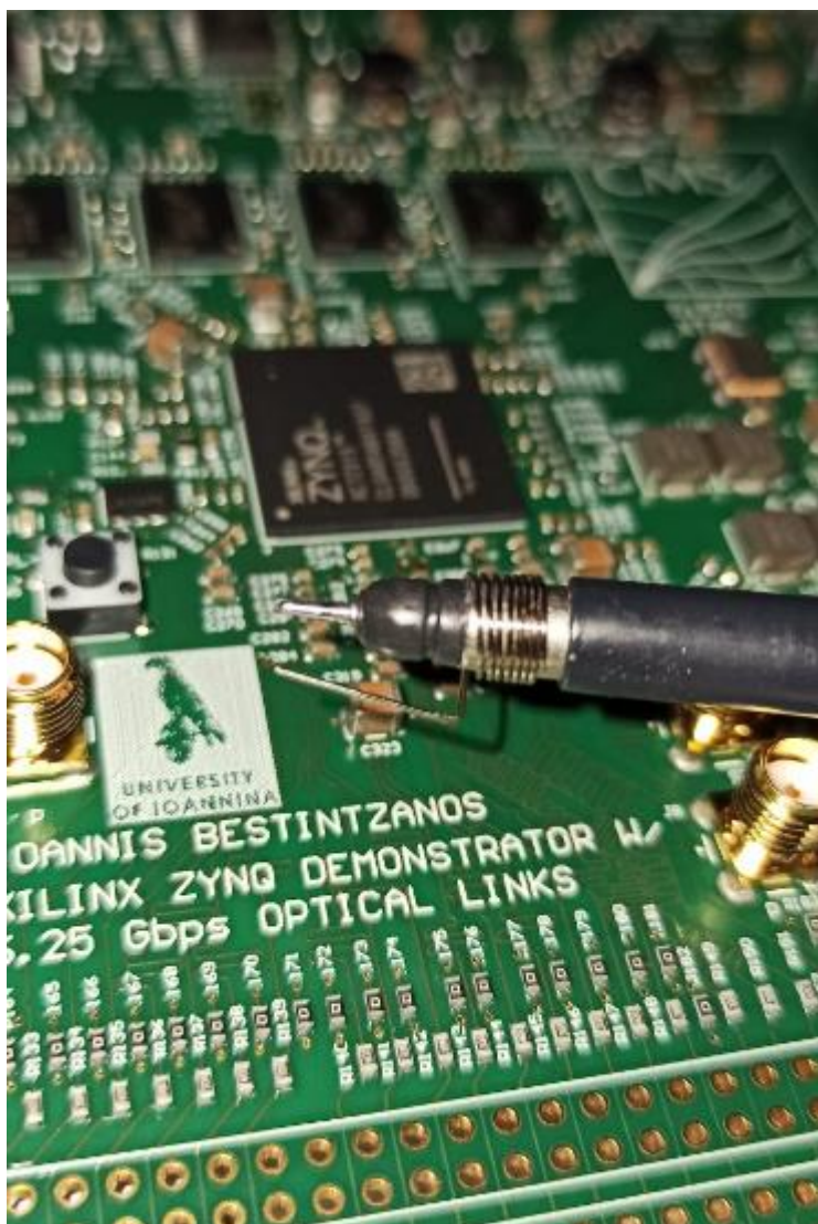
Figure 110. The low inductance ground lead used to probe the power rails.
