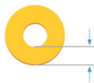
Figure 8. Minimum annular ring.
