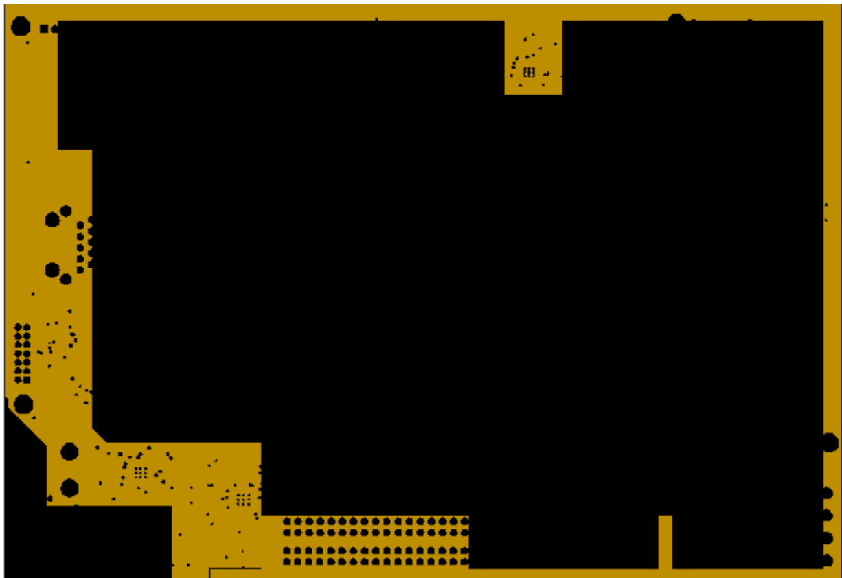
Figure 32. 5V Power plane
