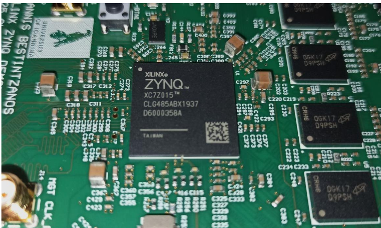
Figure 47. Photo of the ZYNQ device. Visible on the right side is the DDR3 memory.
