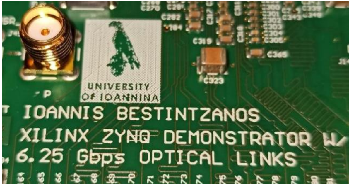
Figure 11. Textures printed on silkscreen. The green layer is the solder mask.
