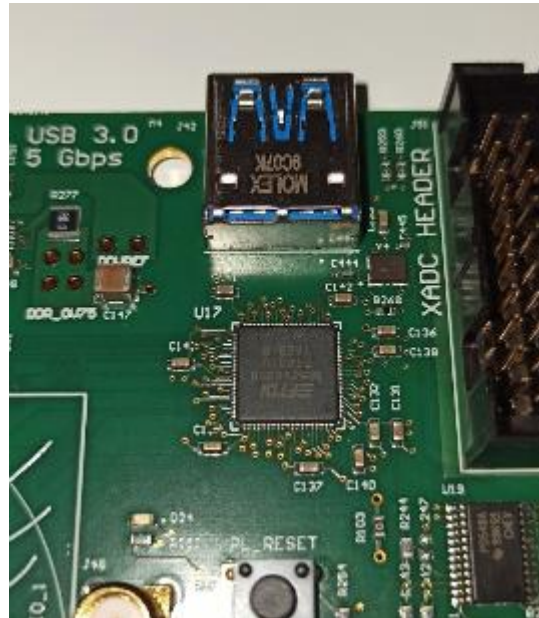
Figure 86. The USB 3.0 circuitry on the board.
