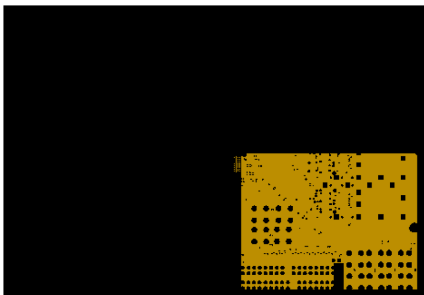
Figure 33. 3.3V plane on power plane 1.
