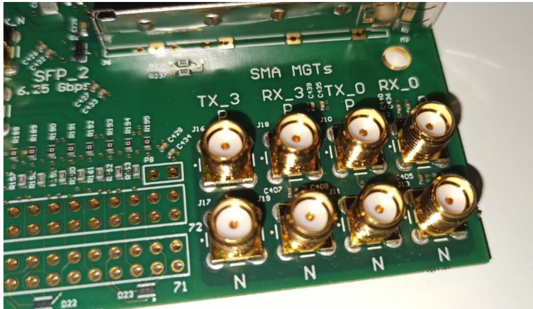
Figure 66. The MGT SMA connectors on the board.
