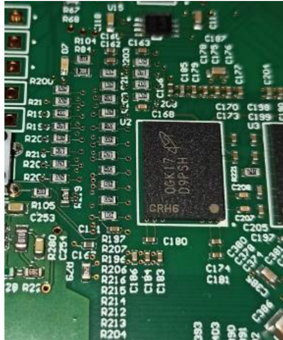
Figure 54. Termination resistors placed right after the last DRAM chip of the Fly-By chain.
