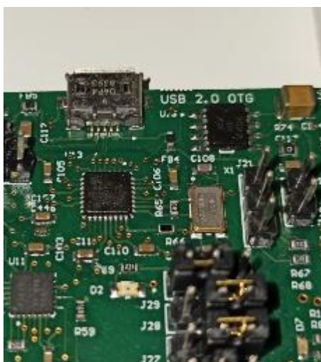
Figure 82. USB 2.0 circuitry on the board.
