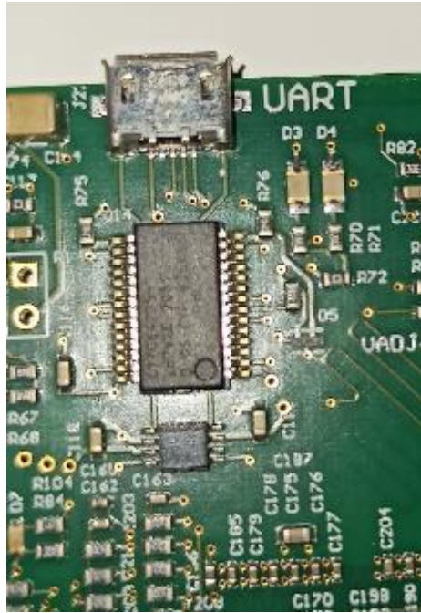
Figure 76. The UART circuit. On the top is the USB-micro connector, in the middle the USB to UART Bridge, and in the bottom the level shifter IC.
