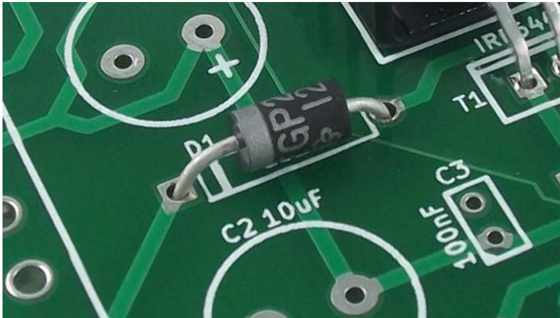
Figure 5. PCB silkscreen and textures showing the polarity of the diode and the electrolytic capacitors.
