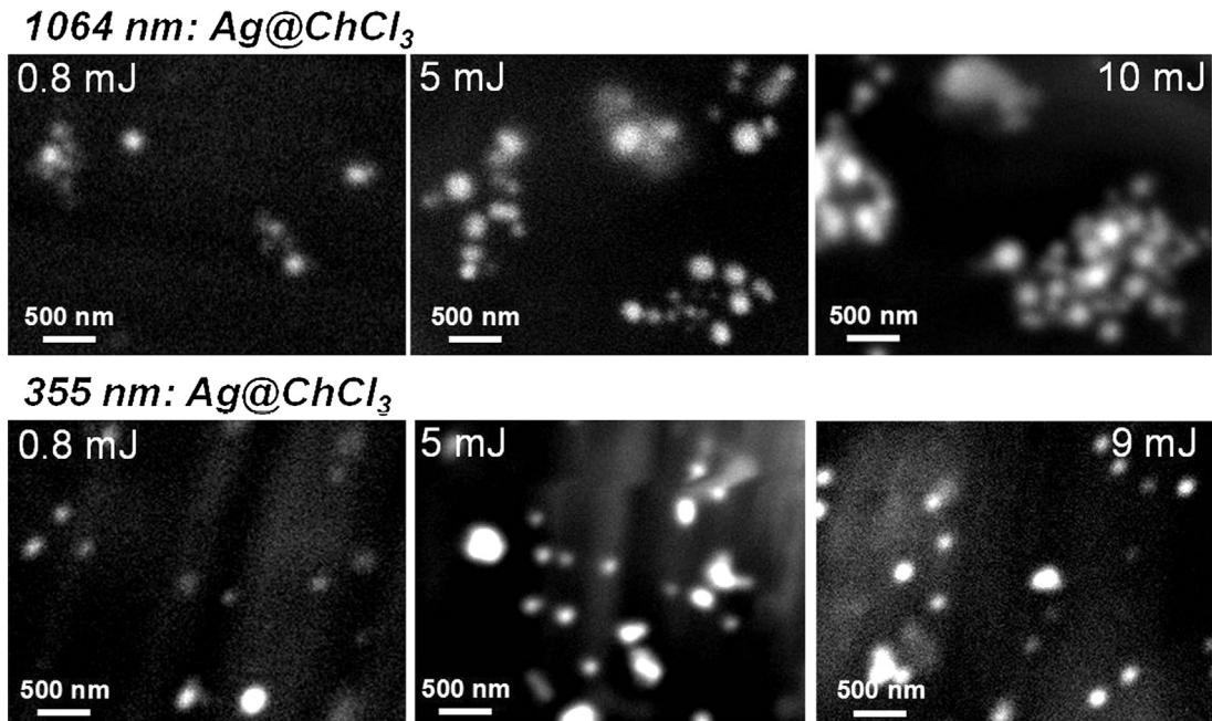
**Fig. 2.** SEM images of the Ag NPs developed in chloroform by laser ablation of a silver target using the 1064 nm and 355 beams of the 35 ps Nd:YAG laser for varying pulse energy.
