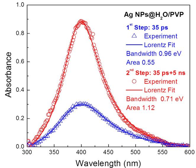
**Fig. 7.** The absorption spectra of the Ag NPs in H<sub>2</sub>O/PVP before (triangles) and after (circles) the size refinement process using an out-of-focus 5 ns laser beam.
