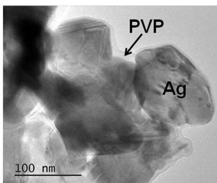
**Fig. 6.** High resolution TEM images show the developed Ag NPs in CHCl<sub>3</sub> solution containing (left) 0.06 mM PVP and (right) 3.7 mM PVP. The LA was made using the 355 nm beam of the 35 ps laser and PE 0.8 mJ/cm<sup>2</sup>.
