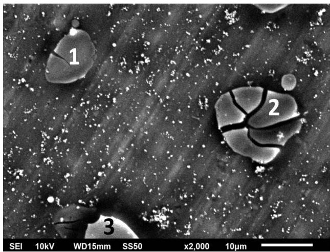
**Fig. 4.** SEM image of the Ag NPs developed in chloroform by laser ablation of a silver target using the 532 nm beam of the 35 ps Nd:YAG laser. The laser power is PE = 10 mJ.
