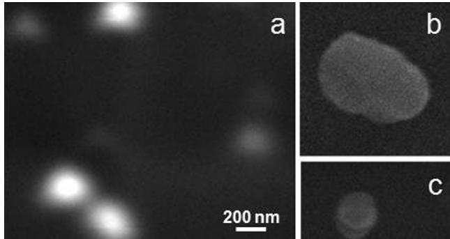
**Fig. 5.** SEM images from (a) Ag@chloroform (355 nm, 10 mJ/cm<sup>2</sup>), (b) and (c) Ag@toluene (355 nm, 10 mJ/cm<sup>2</sup>) colloidal plasmonic solutions. The same scale bar applies to all.
