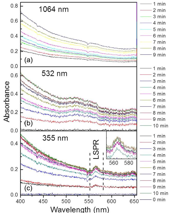
**Fig. 3.** Absorbance spectra for colloidal Ag produced by ps laser ablation in chloroform using three wavelengths (a) 1064 nm, (b) 532, and (c) 355 nm, and various ablation times at 0.8 mJ/pulse. The inset in (c) is a detail of the LSPR feature.
