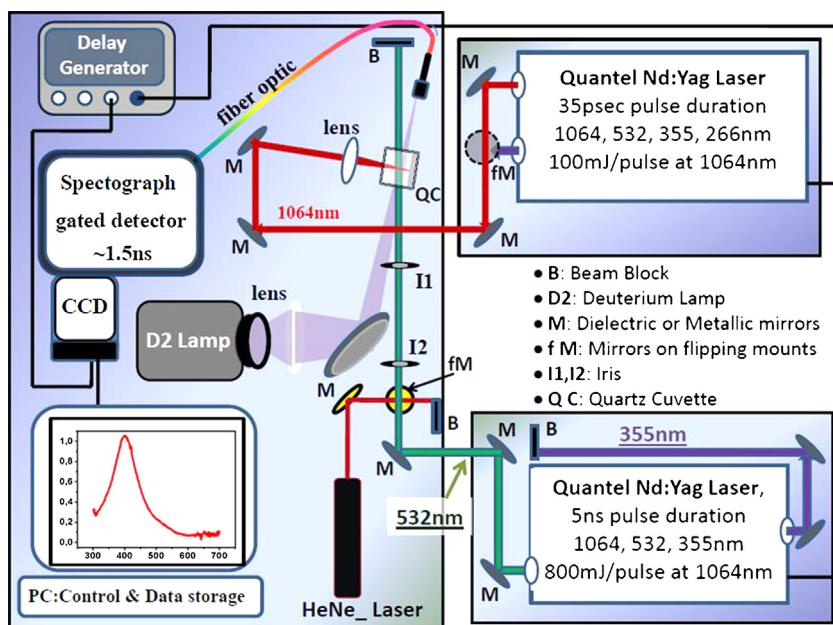
**Fig. 1.** The experimental set up used for laser ablation of the solid target (primary ps laser), laser refinement of particles in the liquid phase (secondary ns laser) and, in situ optical transmittance spectroscopy.
