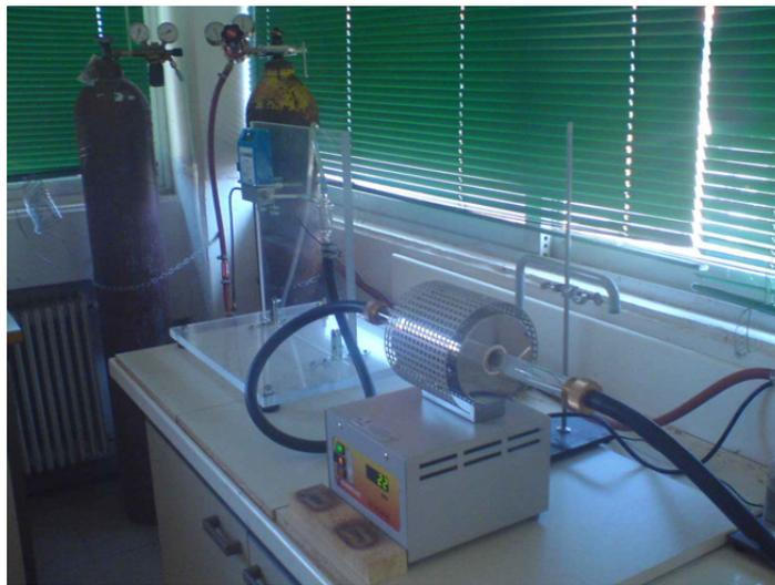
*Figure 22. The horizontal tubular Carbolite furnace used for the CVD process.*
