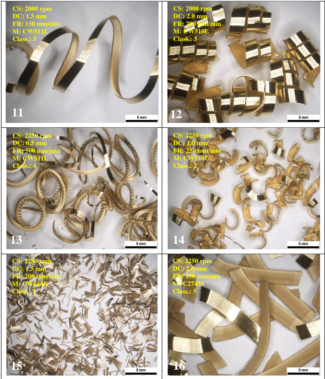
Fig. 3.5: Characteristic forms of Chip Morphology (CM) produced under various turning conditions during the designed experiments (1-16).
