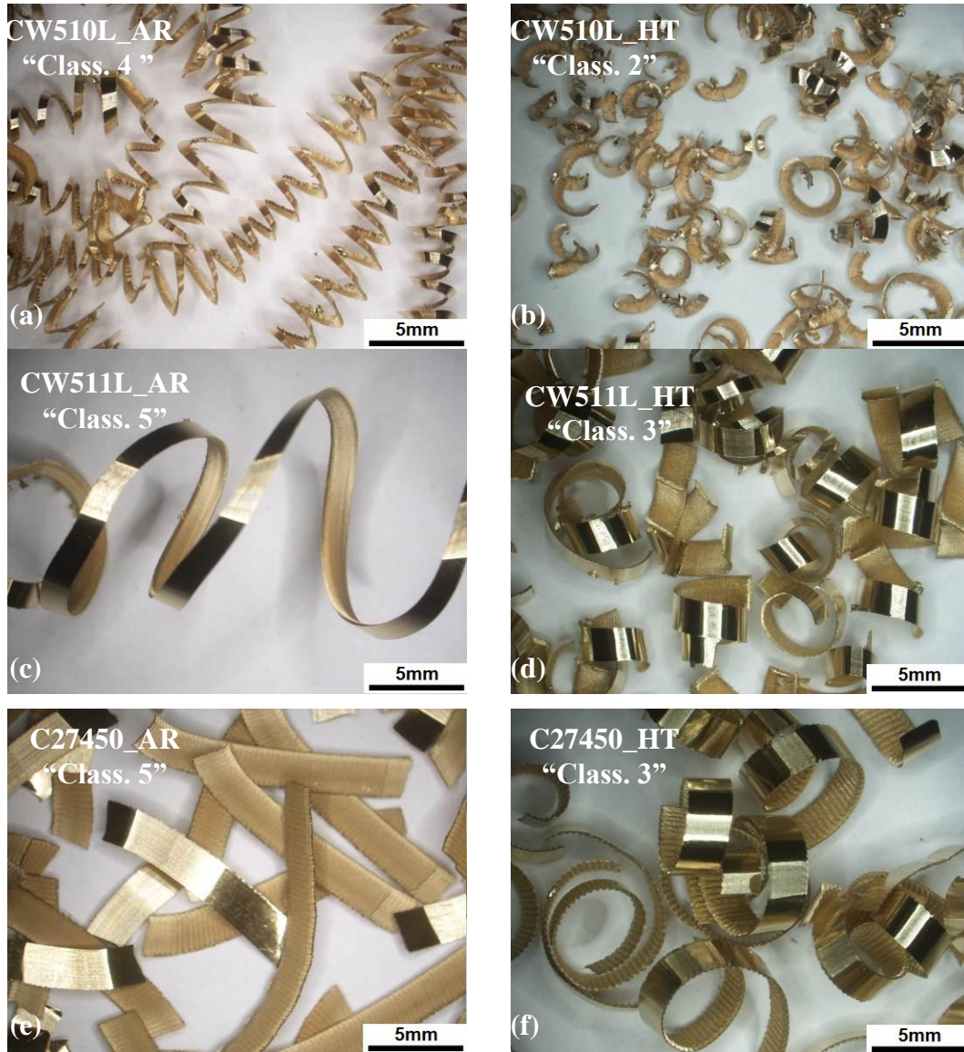
Fig. 7.3: Optimum conditions of chip morphology for the studied alloys after heat treatment (“AR”: as received, “HT”: heat treated). (a) CW510L - as received condition, (b) CW510L – heat treated condition, (c) CW511L – as received condition, (d) CW511L – heat treated condition, (e) C27450 – as received condition, (f) C27450 – heat treated condition.
