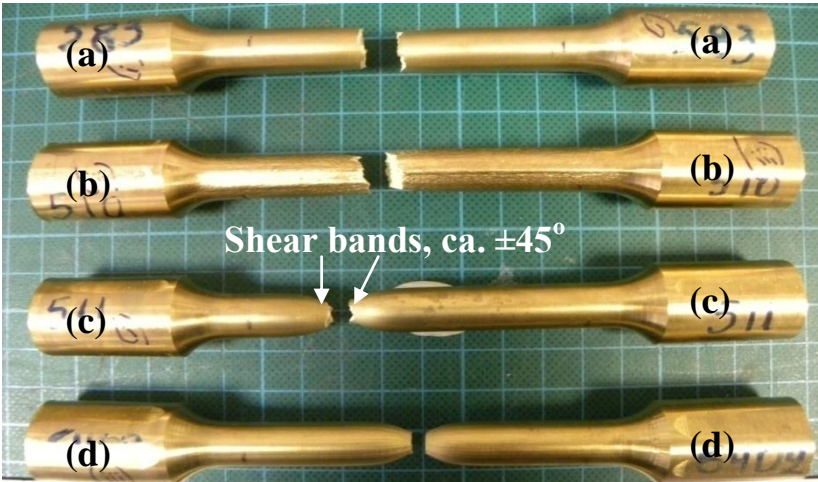
Fig. 2.6: Optical stereomicrographs showing the side view of the tensile fracture surfaces of: (a) CuZn39Pb3 (CW614N) leaded brass as well as (b) CuZn42 (CW510L), (c) CuZn38As (CW511L) and (d) CuZn36 (C27450) lead-free brasses.
