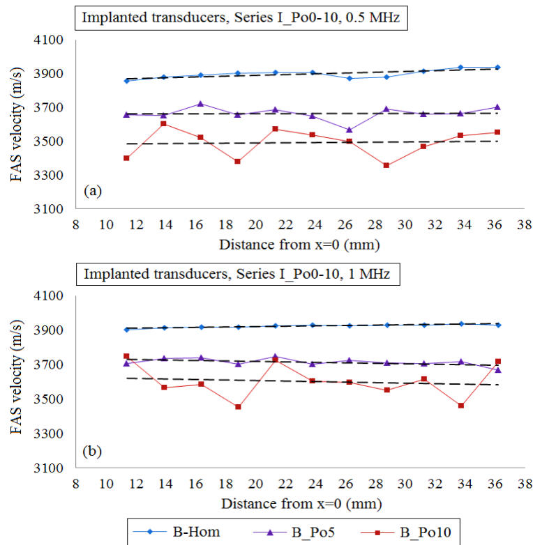
Figure 6.6: Linear fit derived from multiple receiving positions for cortical porosities from 0 to 10%. The diagrams correspond to the first set of simulations under the assumption of implanted transducers and the excitation frequencies: (a) 0.5 MHz, and (b) 1 MHz. The corresponding equations, coefficients of determination and root mean square errors are presented in Tables 6.3, 6.4.
