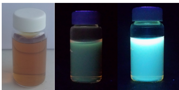
Figure B6. Images of an aqueous dispersion of C-dots with room lights on (left), room lights off but UV illumination on at 254 nm (center) and 365 nm (right).
