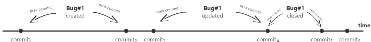
Figure 2 Graphical representation of the method used for linking a bug with the corresponding commits.
