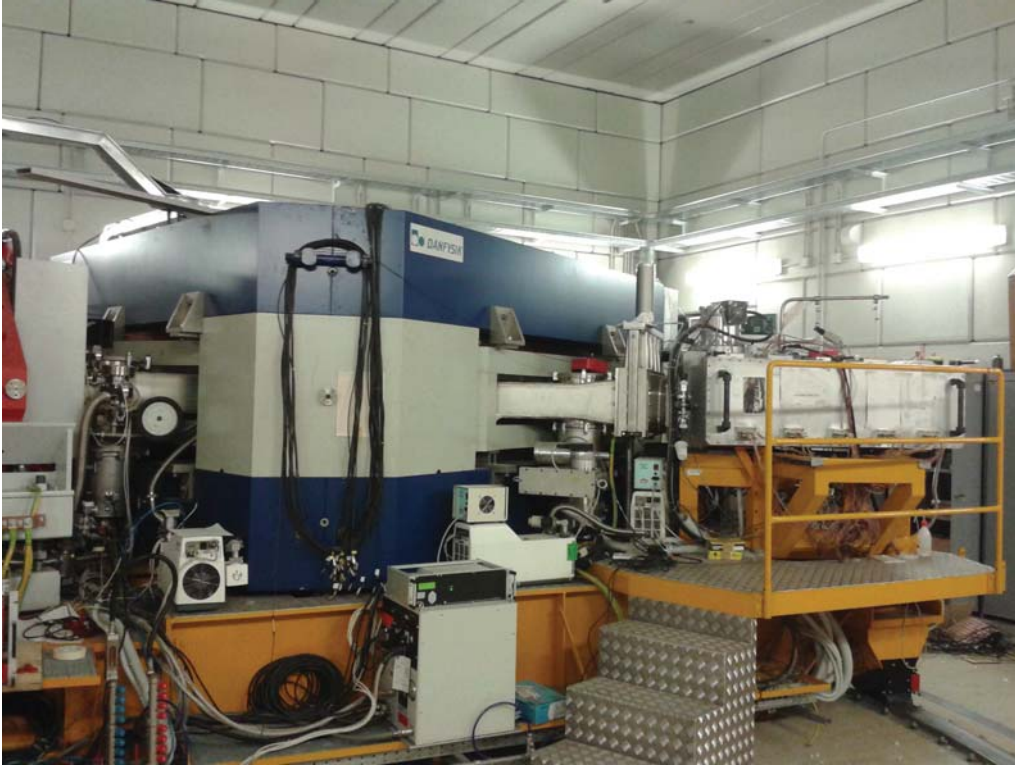
Figure 2.4: A view of the experimental hall with the dipole (center) and the Focal Plane Detector (right).
