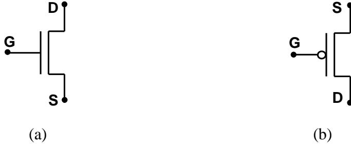
Figure 2.2.: Symbols of NMOS (a) and PMOS (b) transistors
