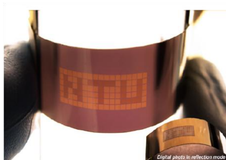
Figure 12. Digital photo of a flexible plasmonic demonstrator capable of optical reading. Photo captured under white light illumination in transmission and reflection (inset) mode. The spots reading 'NTU' were fabricated by LA of the sample with 25 pulses at 15 mJ/cm 2 whereas the surrounding matrix spots were annealed with 1 pulse of 45 mJ/cm 2 . [46]
