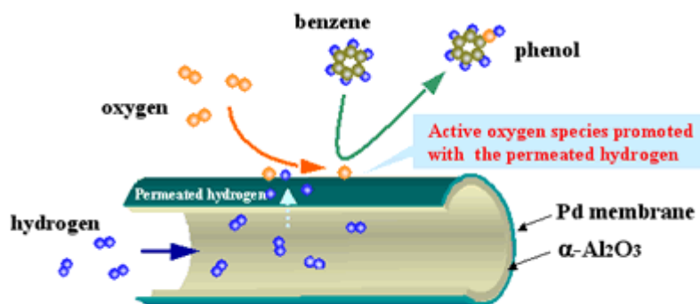
Figure 6. Direct hydroxylation of aromatic compounds by using a Pd membrane reactor
