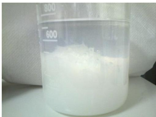
**Figure 4.22:** Image of precipitated  $\text{PI}_{3,4}$  in a large excess of methanol.
