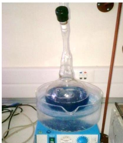
**Figure 4.7:** Picture of the flask with THF in Na/K alloy attached on the vacuum line. The observation of blue color indicates high purity for the specific solvent.
