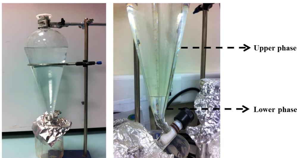
**Figure 4.30:** Images of a separation flask used for the fractionation procedure, indicating the formation of the lower and the upper phase of the mixture (right image).
