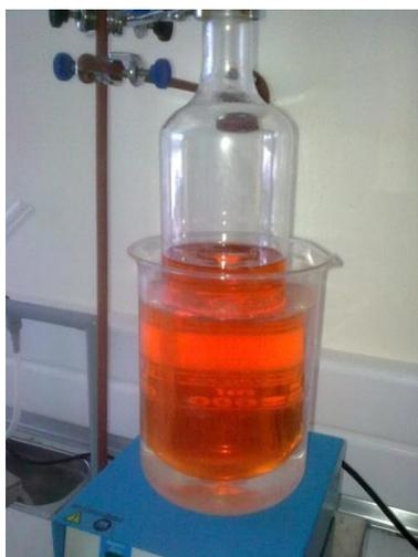
**Figure 4.6:** Picture of a cylinder with (polystyryl)lithium living ends in benzene attached to the vacuum line, indicating the high purity of the solvent due to the orange-red color observed.
