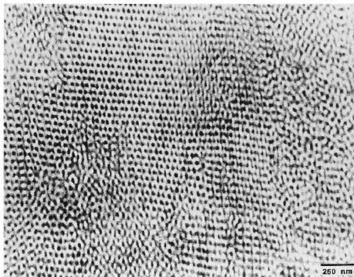
**Figure 3.11:** Bright field TEM micrograph of I<sub>2</sub>S miktoarm star with 53 vol.% PS exhibiting a tricontinuous double gyroid morphology with PI networks (black) in PS matrix (white). The differentiation between the blocks is evident due to staining/cross-linking of the PI domains with vapors of OsO<sub>4</sub> aqueous solution.<sup>95</sup>
