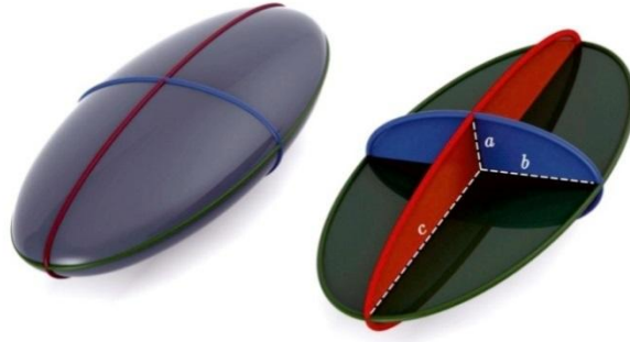
Figure 1.8. A triaxial ellipsoid can lead to three different SPR peaks through to three different axis a, b, c.
