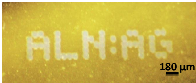
Figure 5.16. The annealed pattern under white illumination. Each pixel of the pattern is approximately 60 \mu m
